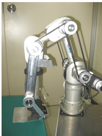
Fig.6.7 The arm for handling tableware
