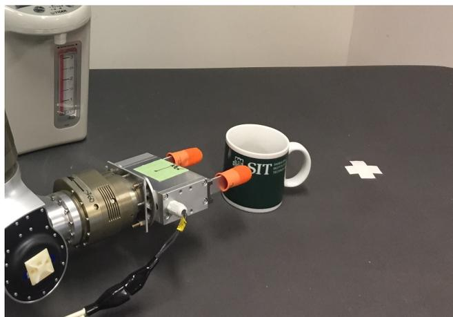
Figure 4.16: The robot arm and hand perform the movement approaching the cup in the situation after recognizing the location and pose of the cup
