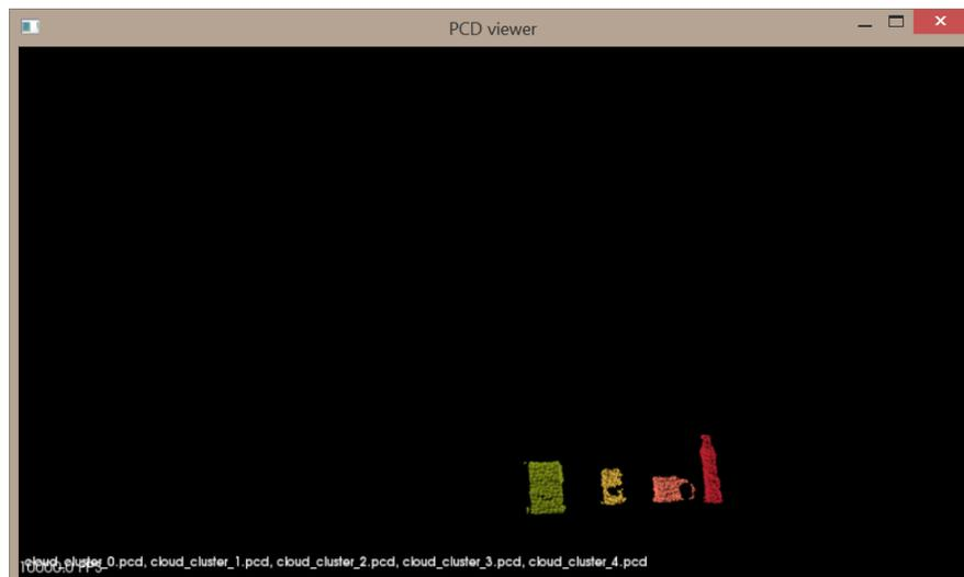
Figure 4.10: Result after planar segmentation and cluster extraction. Four object clusters is segmented and show in one viewer
