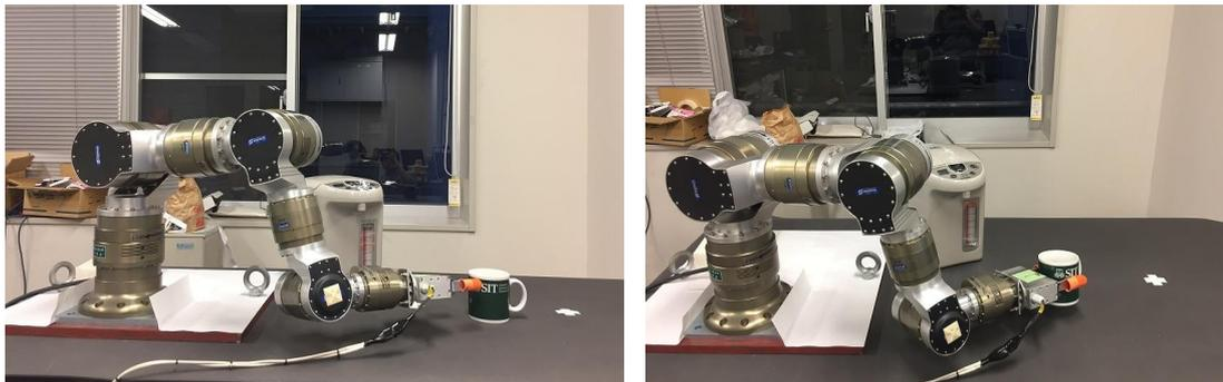
Figure 3.15: Robot arm LWA3 performs the approaching movement to the cup in new location (left photo) and grasping the cup (right photo) with 2-finger hand
