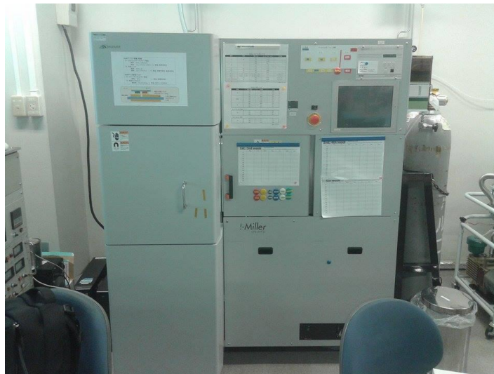
Figure 2.3. The magnetron sputtering set-up in our laboratory (SHIBAURA).
