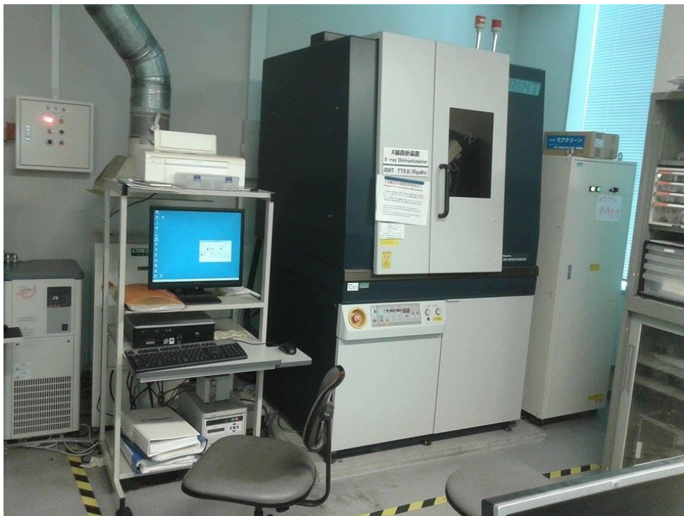
Figure 2.10. XRD measurement system (Rigaku/Rint-TTRIII).
