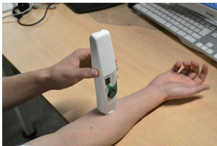
図 6-2. 真皮水分計 (MoistureMeter D Compact, Delfin Technologies Ltd.)
