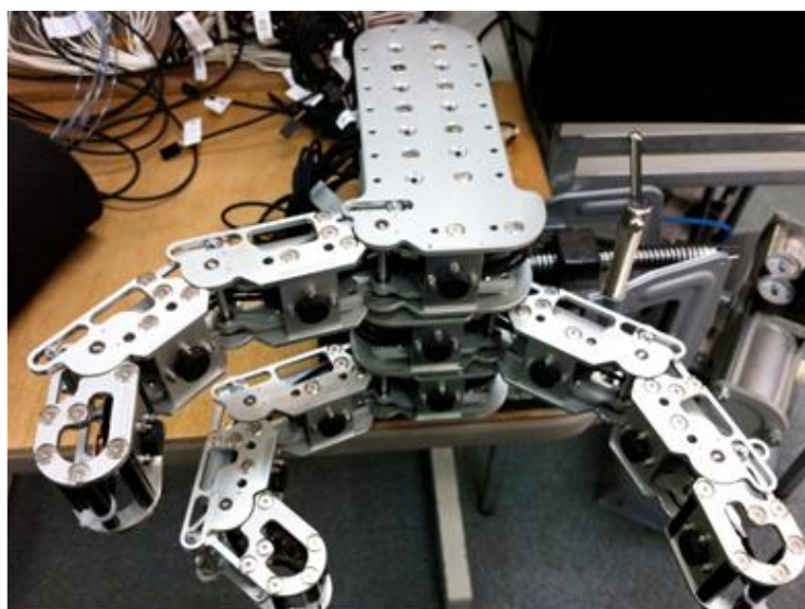
(c) Assembly example of manipulator unit
