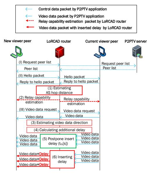
FIGURE 5.4: Time sequence of the LoRCAD Scheme when deployed to P2P application.
