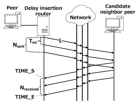
FIGURE 5.6: Relay capability estimation mechanism.
