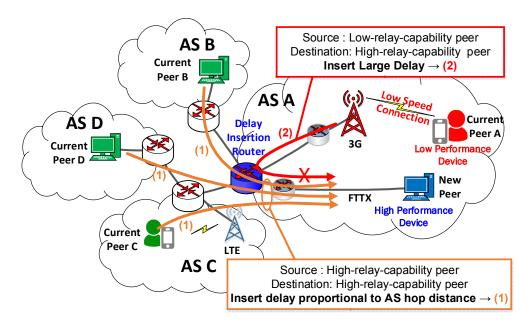
FIGURE 5.2: Operation of the delay insertion router when detecting the high-relaycapability peer.
