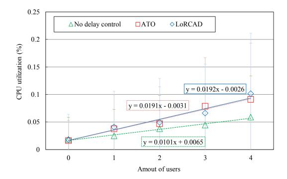
FIGURE 6.15: CPU utilization of delay insertion router with varying the number of viewers.
