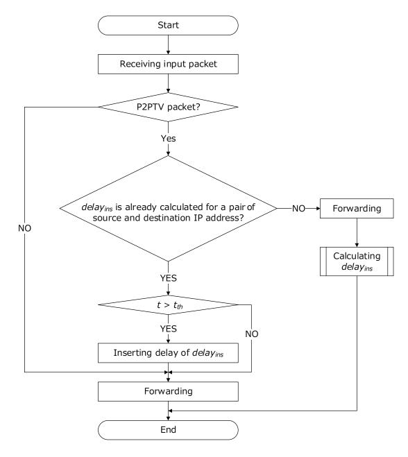
FIGURE 3.3: Flow chart of delay insertion into P2PTV packet by the proposed ATO scheme.
