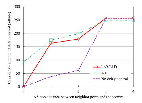
FIGURE 6.6: Cumulative amount of data received by the high-relay-capability peer in SopCast application.
