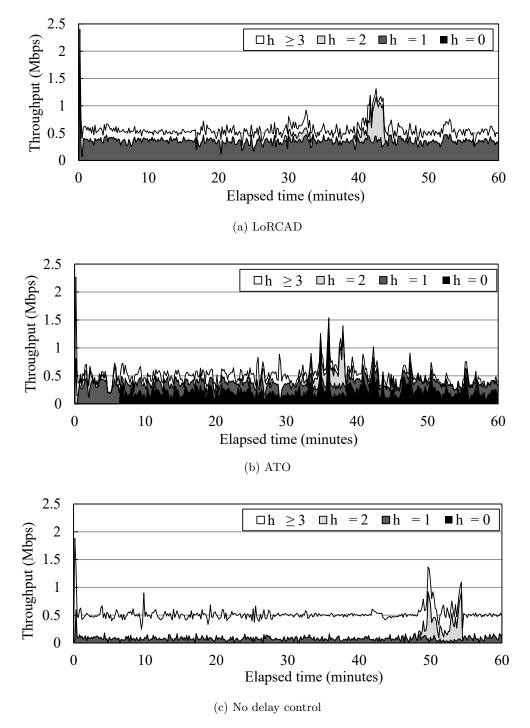
FIGURE 6.7: Download throughput for the high-relay-capability peer in SopCast application.
