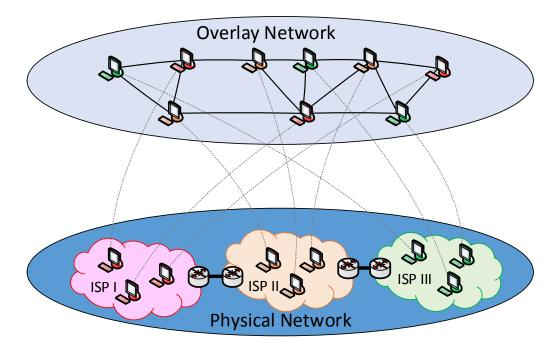
FIGURE 2.6: Connection of peer on overlay network without physical network consideration.
