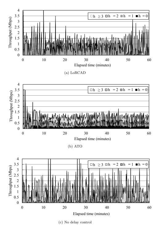
FIGURE 6.9: Download throughput for the high-relay-capability peer in PPLive application.
