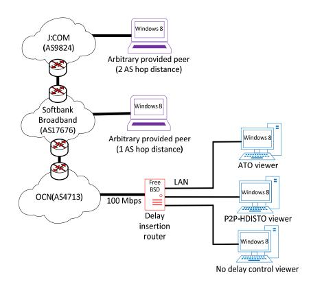
FIGURE 4.1: Experimental setup.
