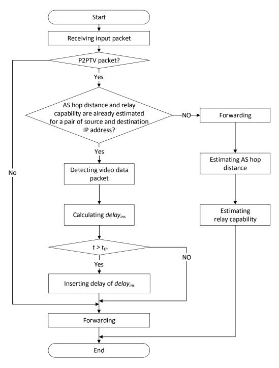
FIGURE 5.5: Flow chart of delay insertion into P2PTV packet by the proposed LoRCAD scheme.
