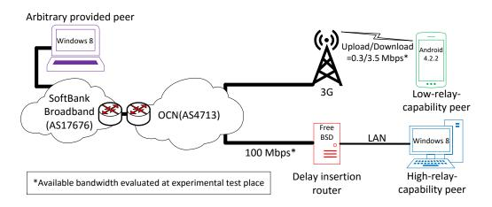
FIGURE 6.1: Experimental setup for LoRCAD scheme evaluation.
