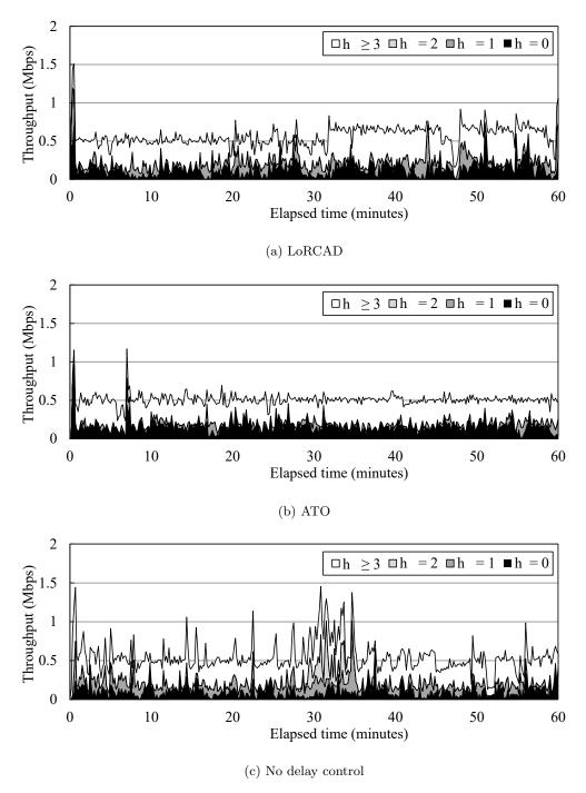
FIGURE 6.11: Download throughput for the low-relay-capability peer in SopCast application.
