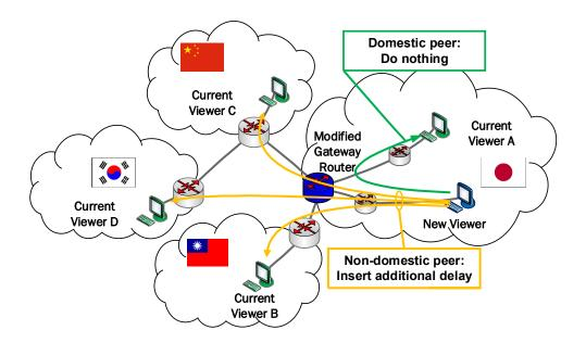
FIGURE 2.11: The concept of P2P-DISTO traffic localization scheme.
