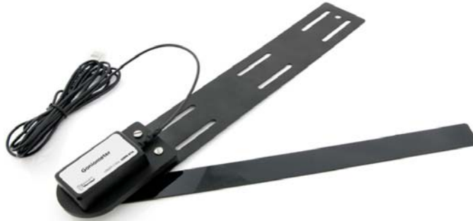
Figure 3: Goniometer - joint angle sensor attached to metal stationary arm
