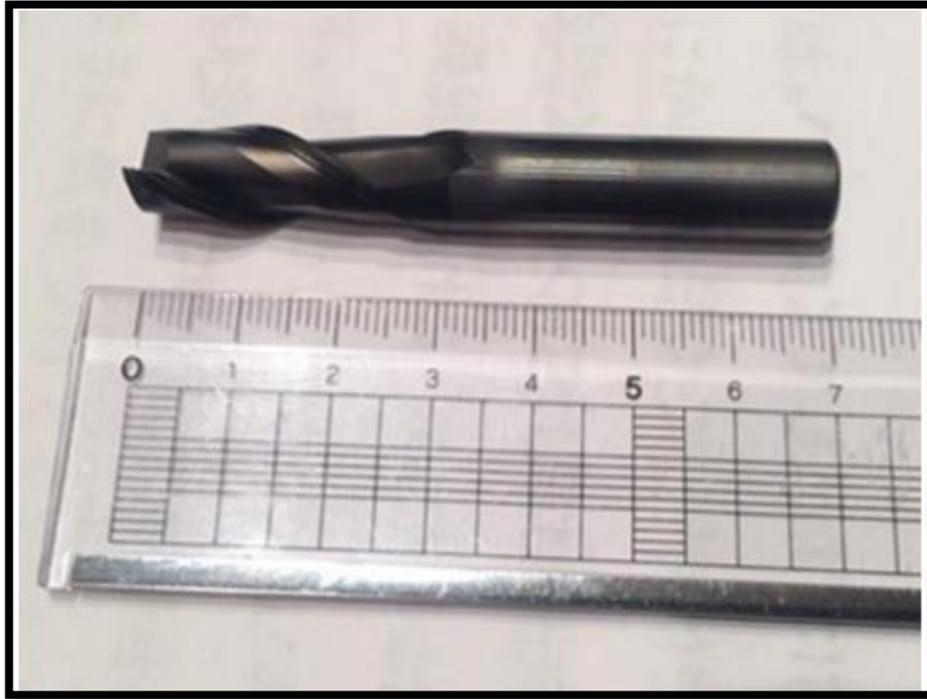
**Figure 2.7 CVD-diamond coated end-milling tools with the film thickness of 15  $\mu\text{m}$**
