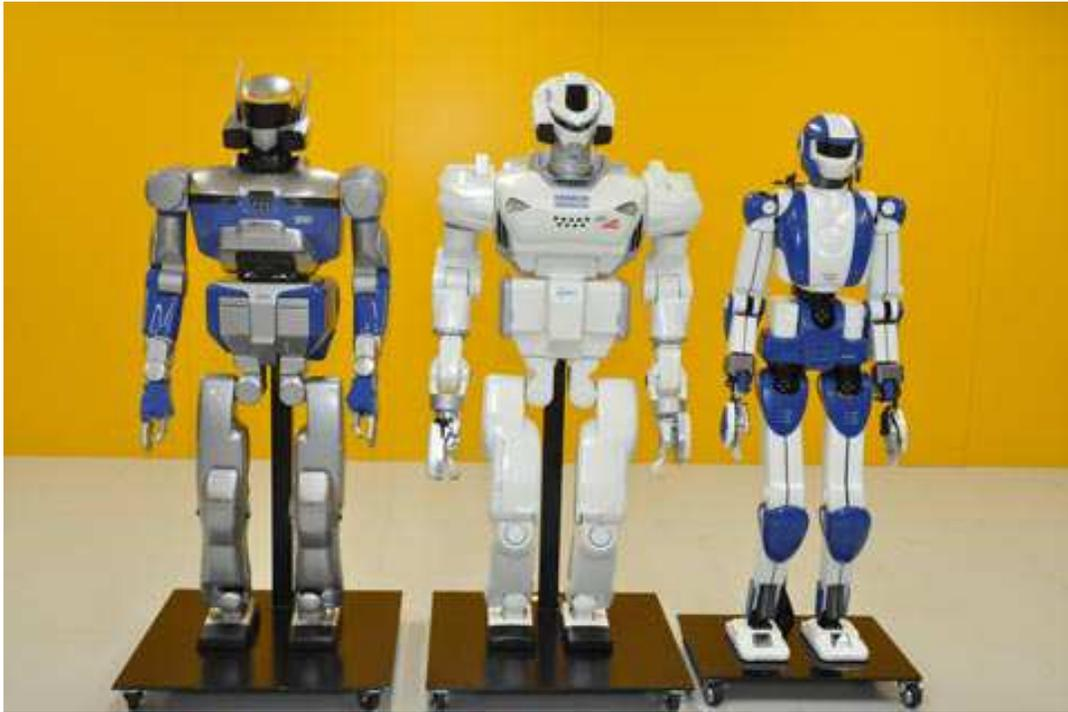
Figure 2.6: The HRP-2, HRP-3 and HRP-4 humanoid robots.
