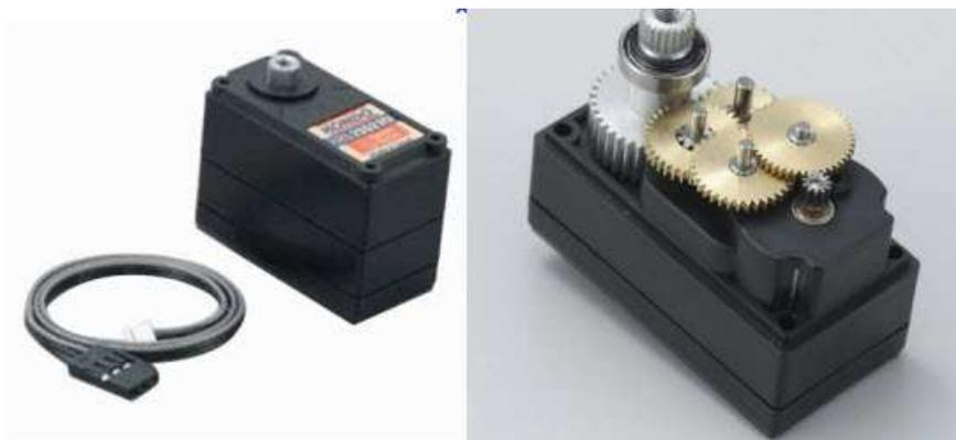
Figure 3.4: KRS-2552HV ICS servo motor red version
