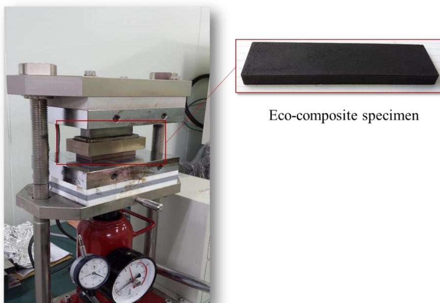
Figure 8 Hot press molding to fabricate specimen.
