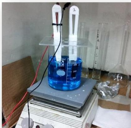
Figure 5.3 Photograph process of electrochemical deposition of copper.
