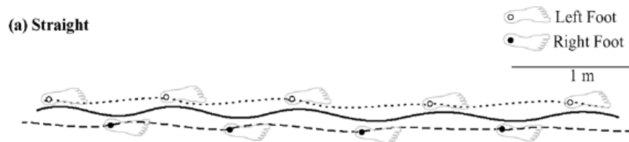
Figure 6.21: The distance trajectory ( X_d ) and foot of model B2 compare with human [43]
