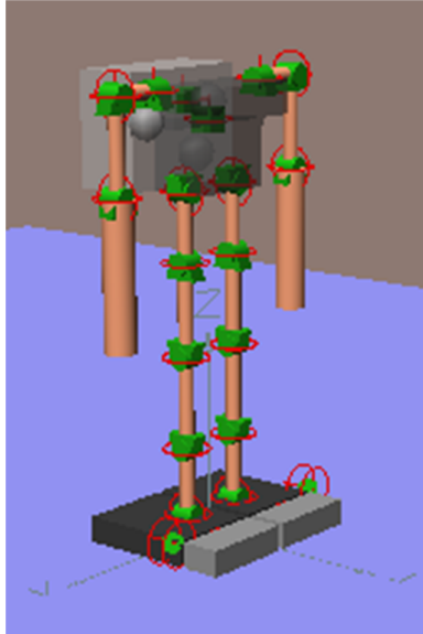
Figure 5.1: The simulation model is made from MSC. Visual Nastran Desktop 4D on flat grounds (FG)
