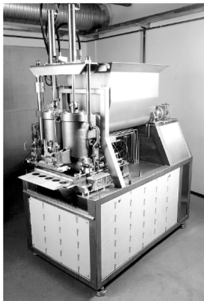
Figure 1.7: Tap water hydraulic driven burger-machine [1].
