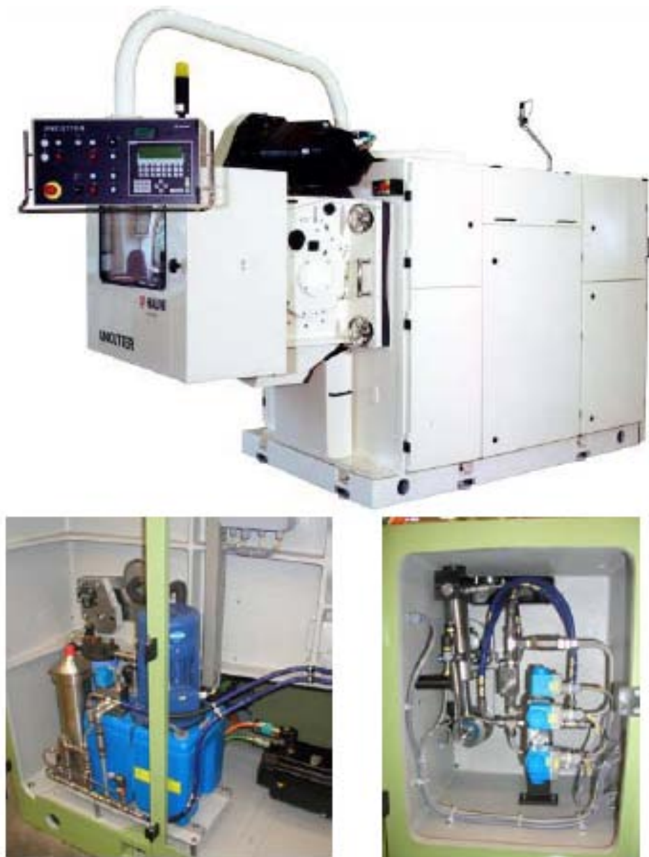
Figure 1.9: Automatic control tobacco cutter machine driven by water hydraulics with two cylinders [1].
