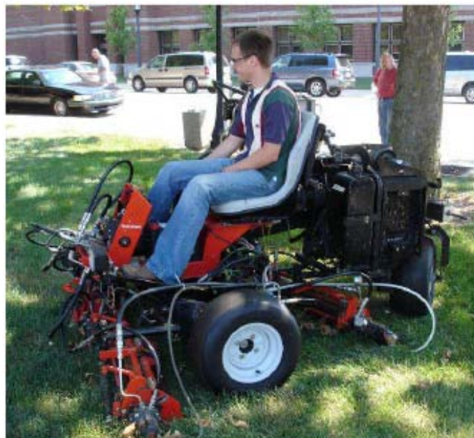
Figure 1.4: Self-propelled water hydraulic vehicle [2].
