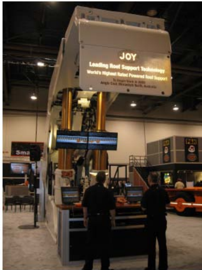
Figure 1.5: 1750 ton roof support with 480 mm bore leg cylinder – note the bronze plated rods [3].
