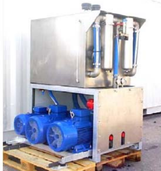
Figure 1.10: Water hydraulics drives for wing press equipment for an aero plane factory [1].
