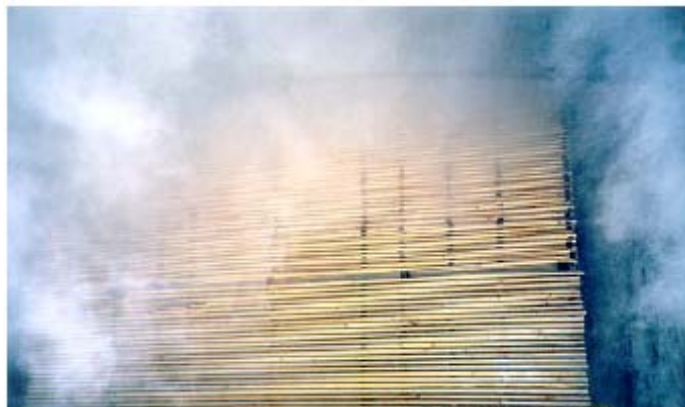
Figure B.5: control Process for lumber drying in a kiln [1].
