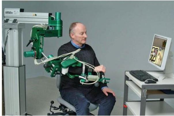
Figure 2 : Rehabilitation Robot ARMin
