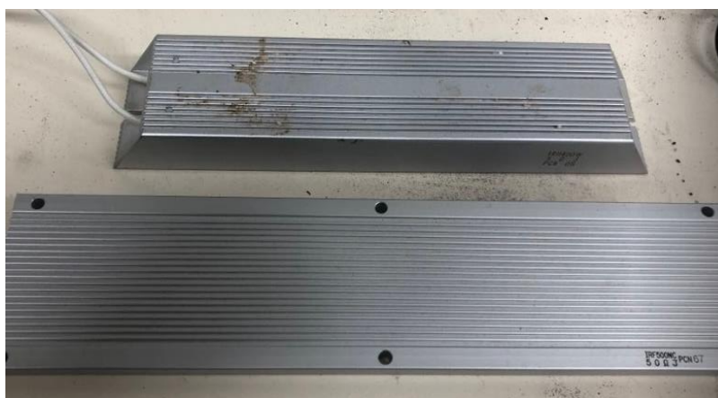
Figure 2.7: The top wirewound resistor has value of 25Ω and the bottom one has value of 100Ω.
