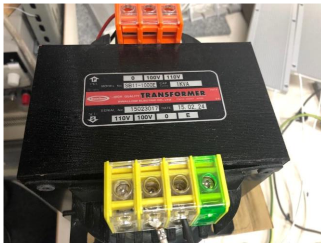
Figure 2.6: Isolation transformer used in the main experiment.
