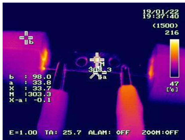
Figure 4.4: Heat generated from 4.00A Arc-fault, 4 minutes later.
