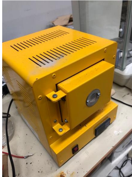
Figure 2.2: Furnaces used in the experiment to temper the copper metal.
