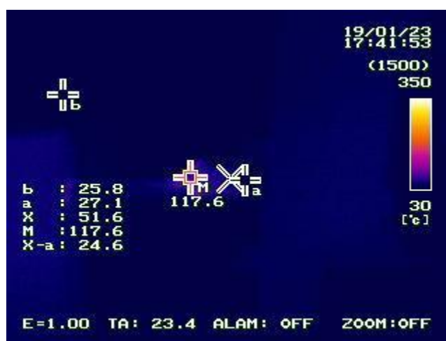
Figure 4.11: Heat generated from 4.00A Arc-fault initial state.
