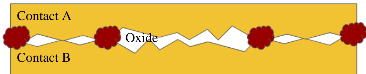
Figure 7.4: Oxides is formed around the contact points.
