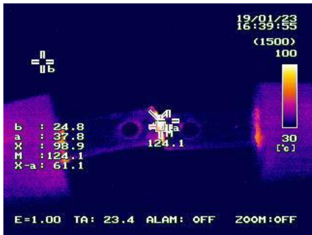
Figure 4.8: Heat generated from 8.33A Joule heating.
