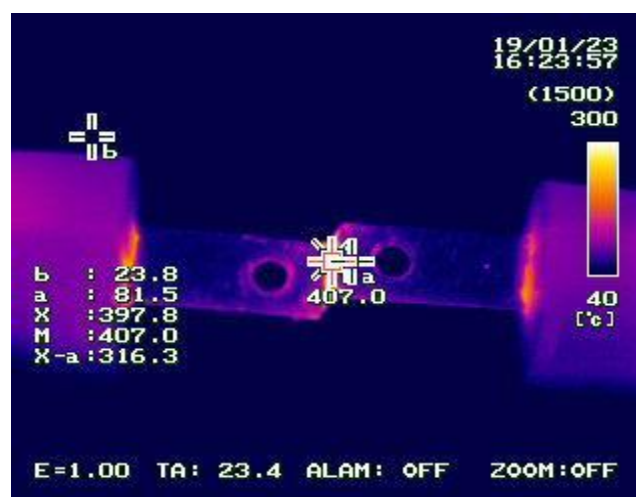
Figure 4.7: Heat generated from 8.33A Arc-fault, one minute later.
