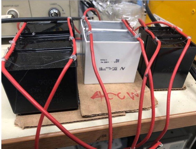
Figure 8.2: Array of capacitors used to power correct the phase shifted.
