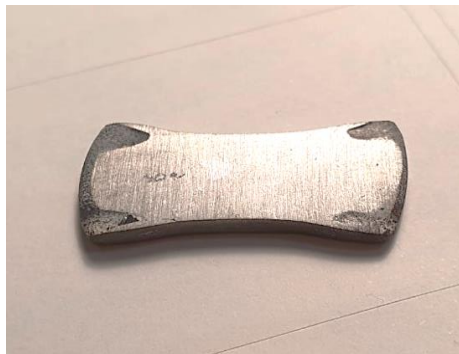
Figure 29 - Skutterudite sample after ODP pressing ( \approx 3 cm long). It is noticeable the dog-bone shape of the resulting dense sample.
