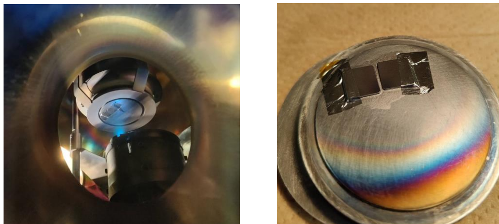
Figure 55 - (on the left) Bottom view of the samples in the chamber. They are glued upside down. (on the right) Samples after the deposition. The Kapton tape and the position on the holder are visible.
