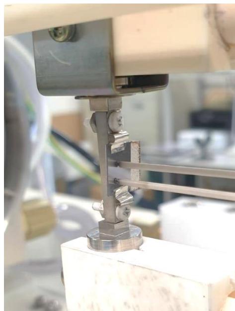
Figure 40 - On the left, side view of the experimental custom-made set-up for the thermoelectric properties' measurement of thin films. On the right, a picture of skutterudite thin film on the special holder is shown.
