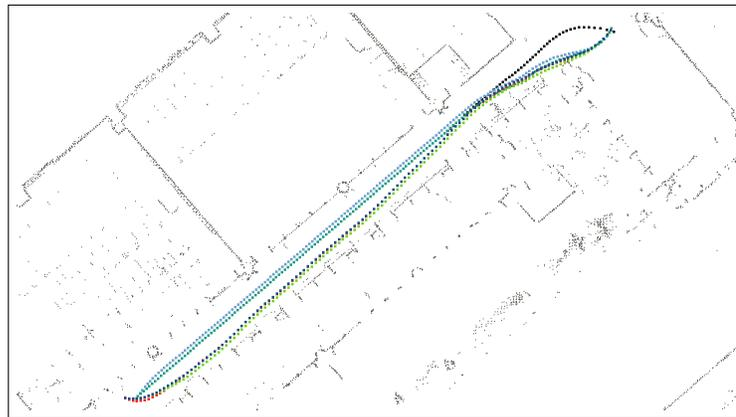
(b) The trajectories from 4.7(a) on point cloud map. Red(non augmented results of both A\* and APF\*) Green (augmented result of both APF and A\*)
