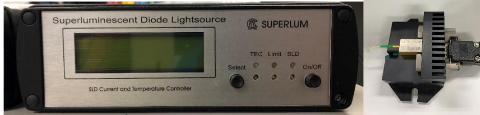
Figure 4.1 Superluminescent diode emitting broadband light wave at 1550 nm.
