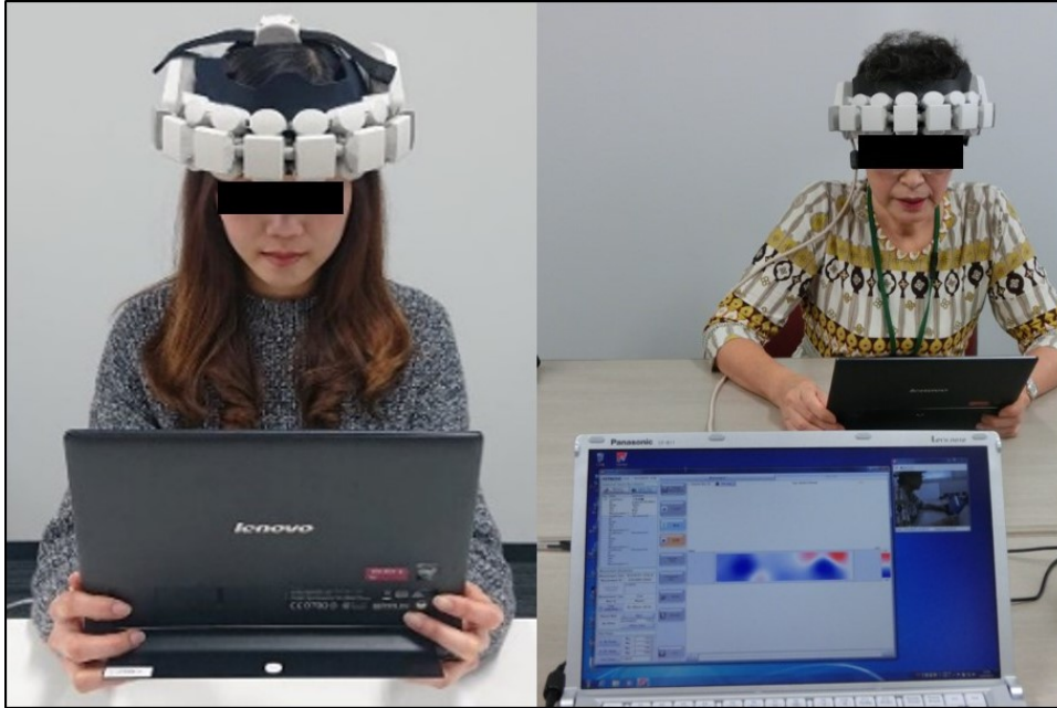
FIGURE 5.8: Positions of NIRS WOT-100 probe on the subjects' head
