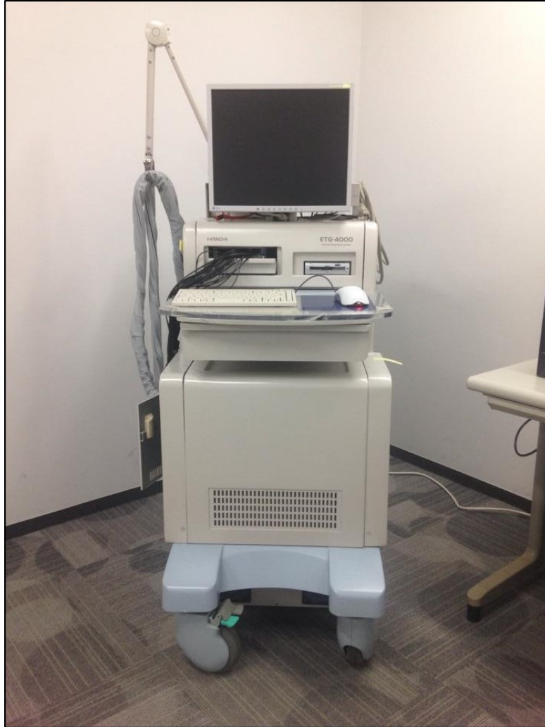
FIGURE 3.2: Image of the NIRS system (ETG-4000) used in this study
