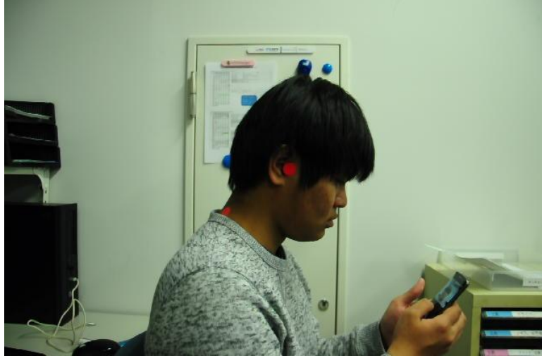
FIGURE 4.10: Positions of two red stickers for photogrammetric method for neck angle measurement
