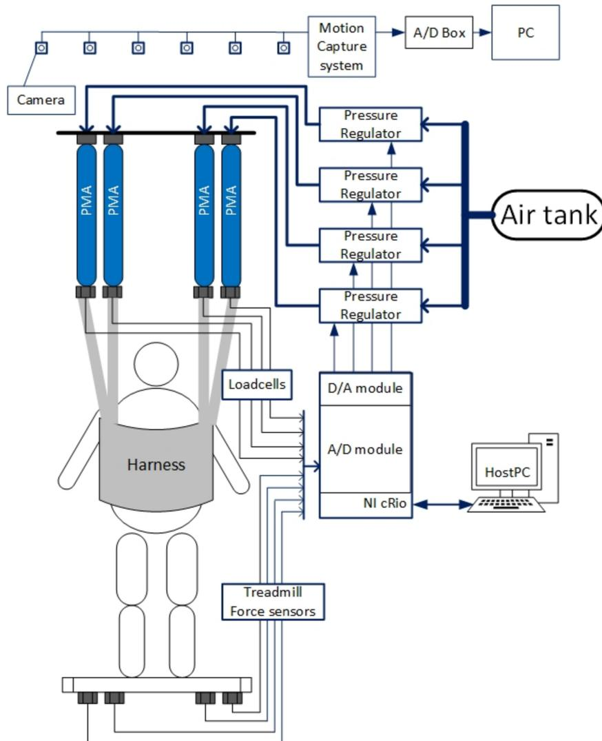
Figure 3.1: Scheme of the BWS system using pneumatic muscle actuators is represented.
