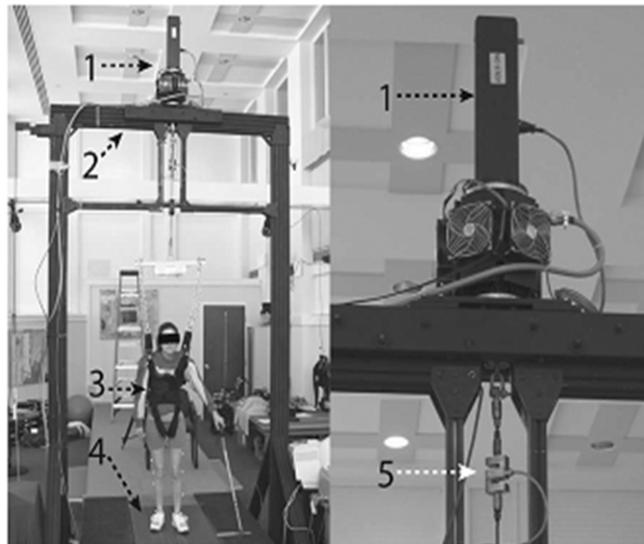
Figure 1.4: A BWS system using electrical motor [29].
