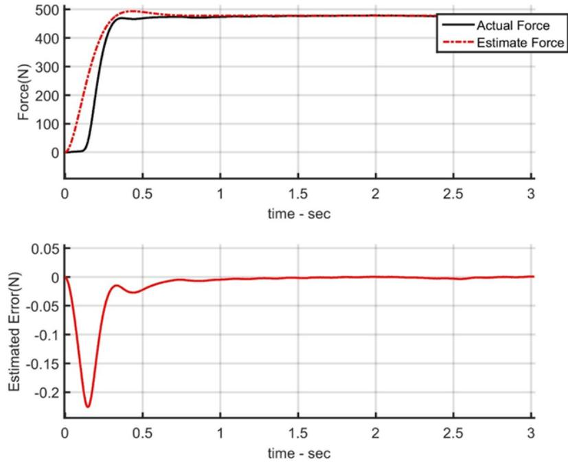
Figure 4.1: Step response of the model and the actual system.
