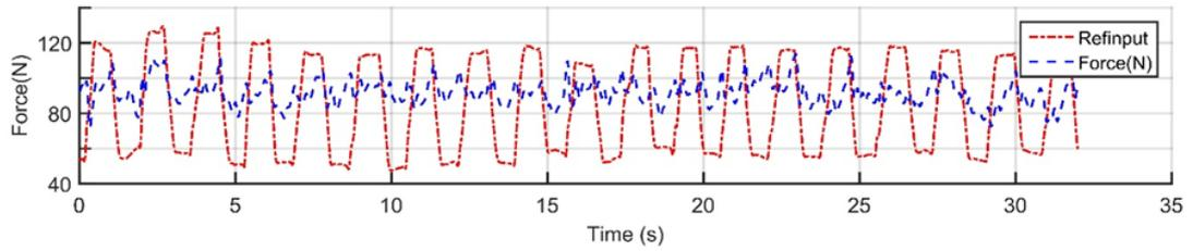
Figure 5.11: The adaptation of the unloading force for the Counter Weight system on the left side. The red line represents for desired unloading force (named Refinput), the blue line represents the actual force.
