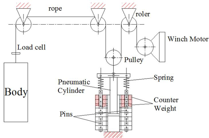
Figure 3.3: Scheme for the first idea of the active BWS system which combines the pulley-rope mechanism and the counter weights.
