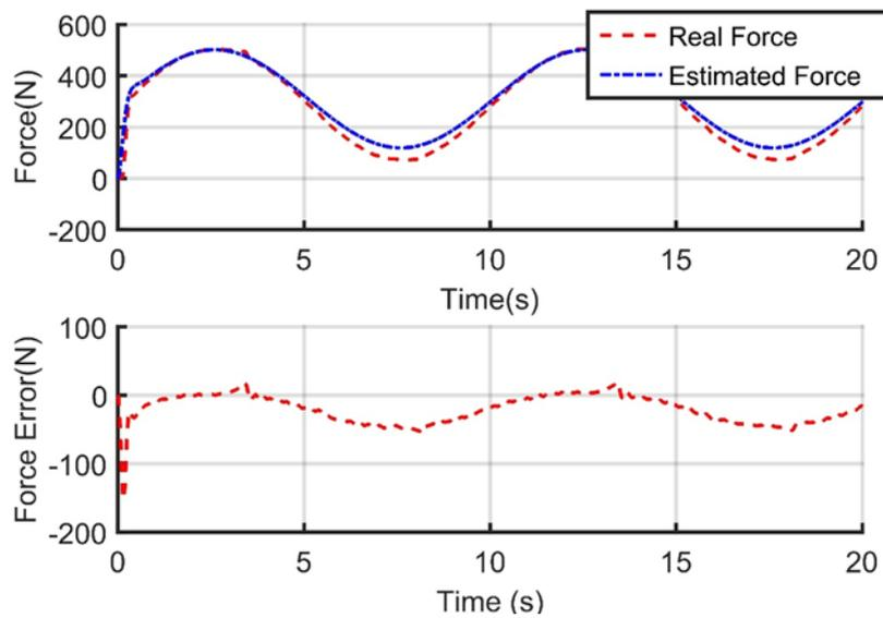
Figure 4.2: Comparison between the estimated force from model and the measurement force from muscle at frequency 0.1 Hz.
