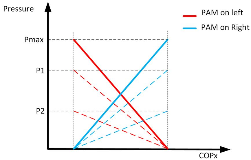
Figure 4.7: Demonstration of changing the instantaneous value of pressure in PAMs.
