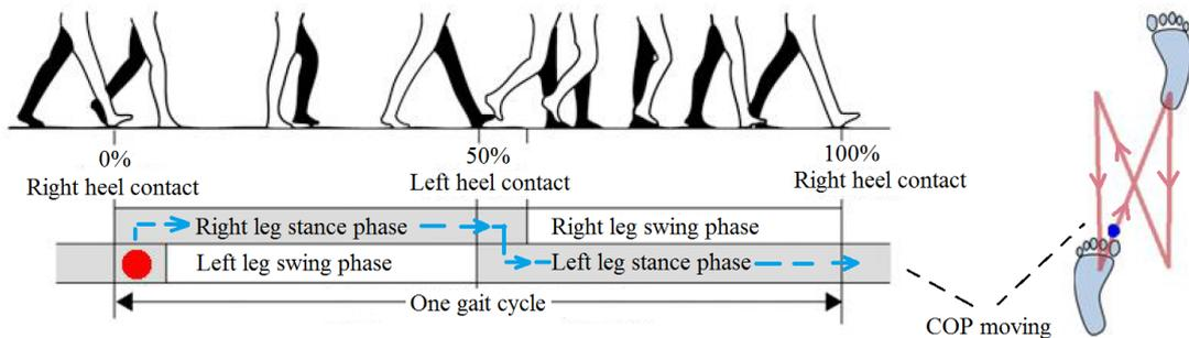
Figure 4.5: Demonstration of COP moving in force plate.
