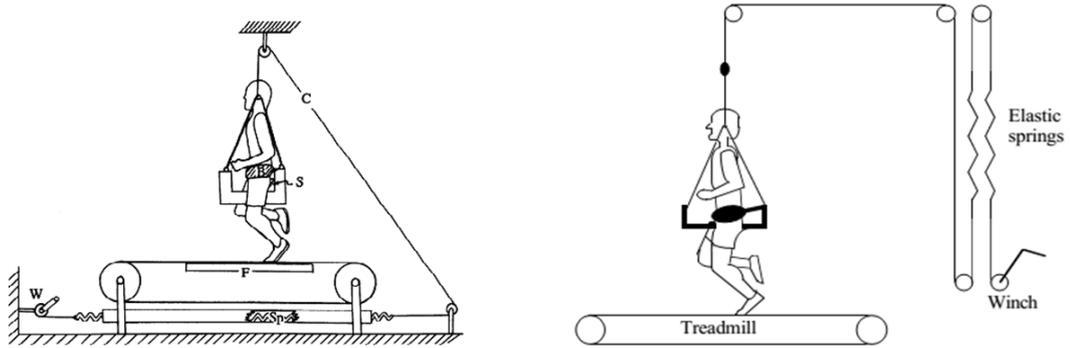
Figure 1.1: Scheme of BWS apparatus using series of springs [30] [18].
