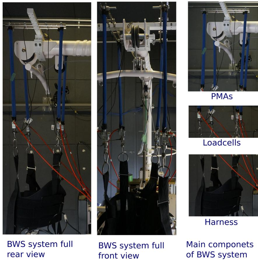
Figure 3.2: The prototype of the new BWS system.
