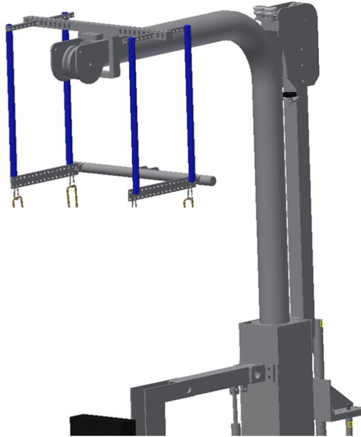
Figure 3.7: The new design for BWS system using four pneumatic muscle actuators.
