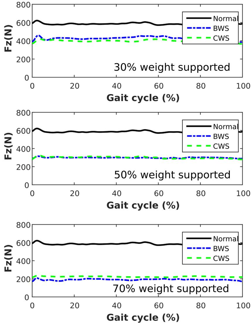
Figure 5.7: Reaction Force in one Gait Cycle the black line represents for the normal walking, the blue line represents for BWS system, and the green line represents for Counter Weight system. From the top to the bottom, the weight support level is 30%, 50%, and 70%, respectively.
