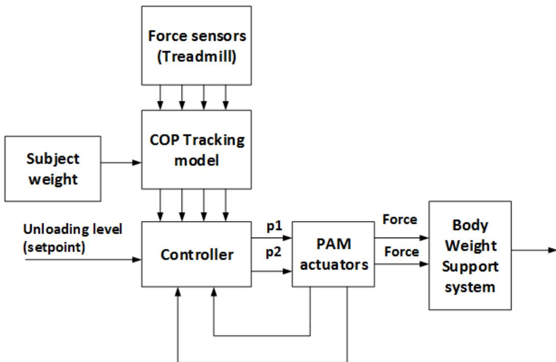
Figure 4.8: Block diagram of proposed tracking COP movement control model.
