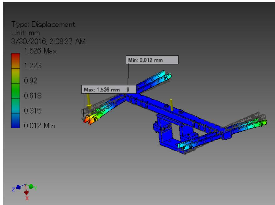
Figure 3.10: The maximum displacement is reached to 1.5 mm.
