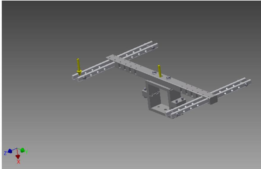
Figure 3.8: The most dangerous case since all load concentrate at the furthest position.
