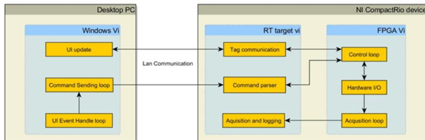
Figure 4.10: The main blocks of software program based LabVIEW using for controlling the BWS system.
