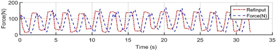
Figure 5.10: The adaptation of the unloading force for the BWS system on the left side. The red line represents for desired unloading force (named Refinput), the blue line represents the actual force.
