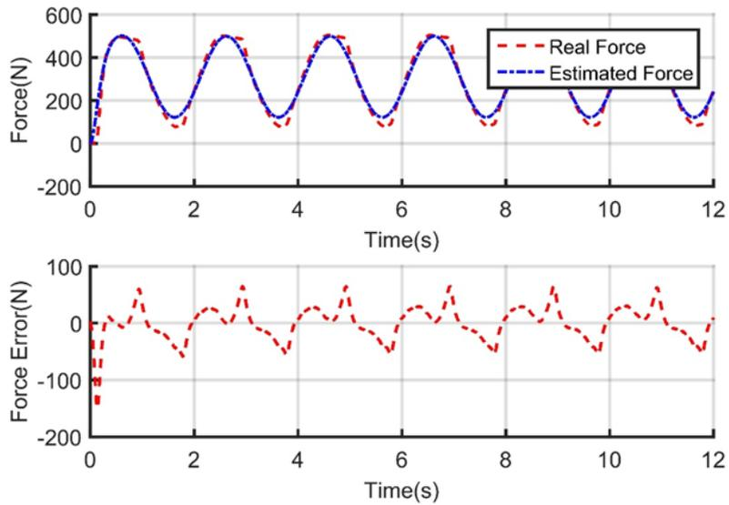
Figure 4.4: Comparison between the estimated force from the model and the measurement force from muscle at frequency 0.5 Hz.
