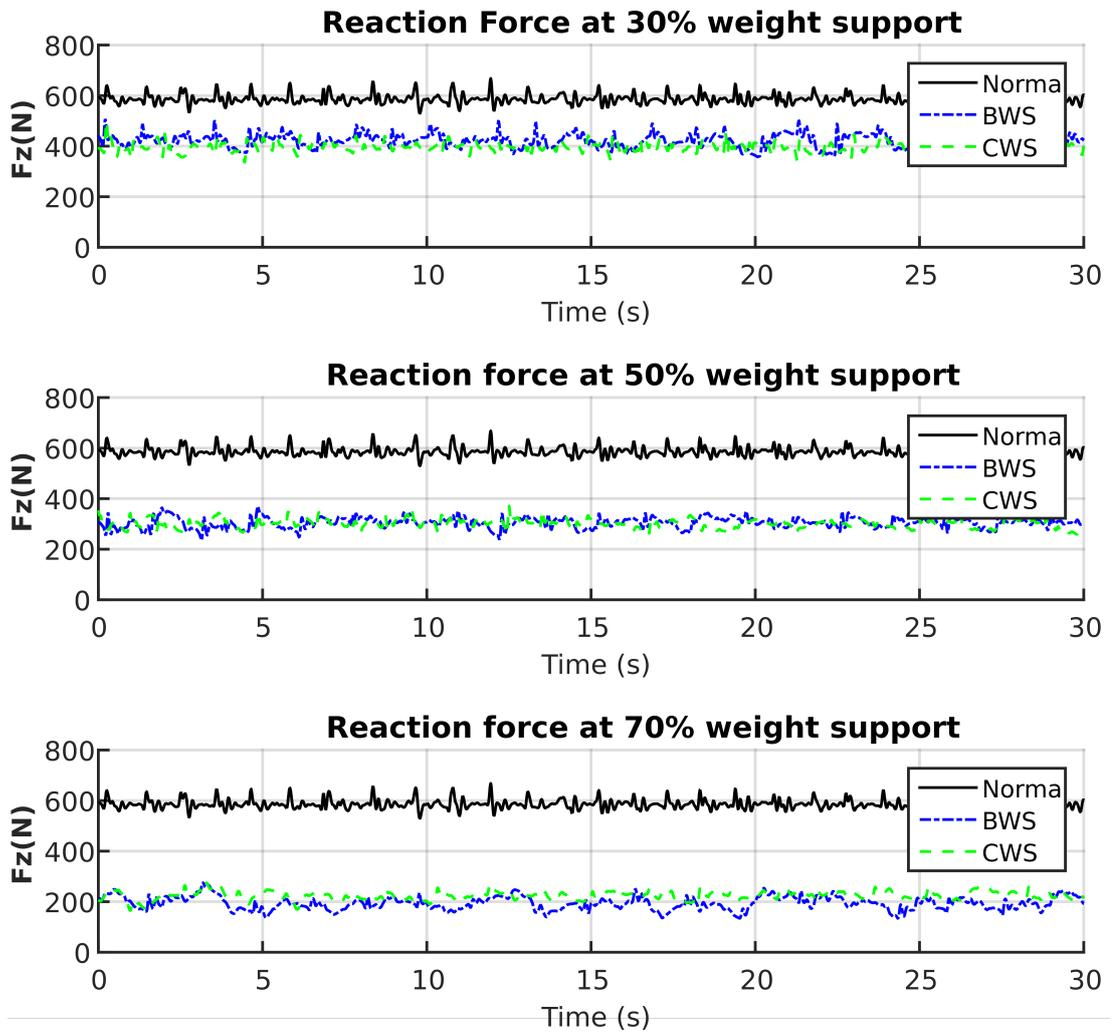
Figure 5.6: Reaction Force When applying BWS system. The black line represents for the normal walking, the blue line represents for BWS system, and the green line represents for Counter Weight system. From the top to the bottom, the weight support level is 30%, 50%, and 70%, respectively.
