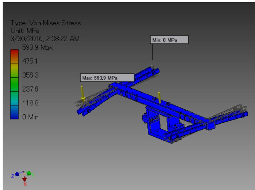
Figure 3.9: The Dynamic Simulation result in which the maximum Von Mises stress reach to 593 Mpa is represented.
