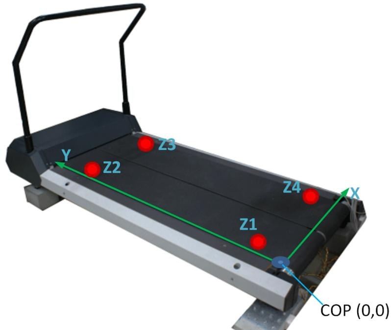
Figure 4.6: Treadmill with four force sensors integrated into four corners.
