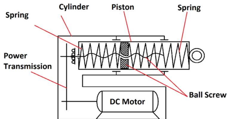
Figure 3.6: Principle scheme of the Linear elastic actuator.
