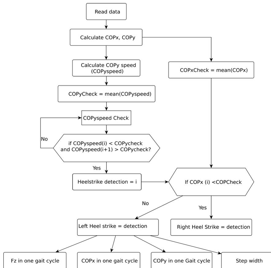
Figure 5.1: The procedure to calculate vertical ground reaction force (Fz) and COP movement.
