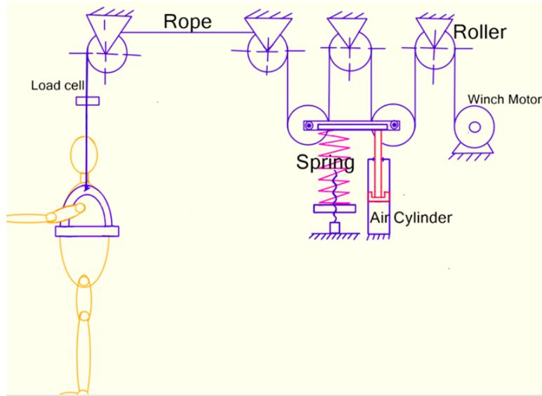
Figure 3.4: Scheme for the second idea the active BWS system which combines the pulley-rope mechanism, spring and air cylinder.
