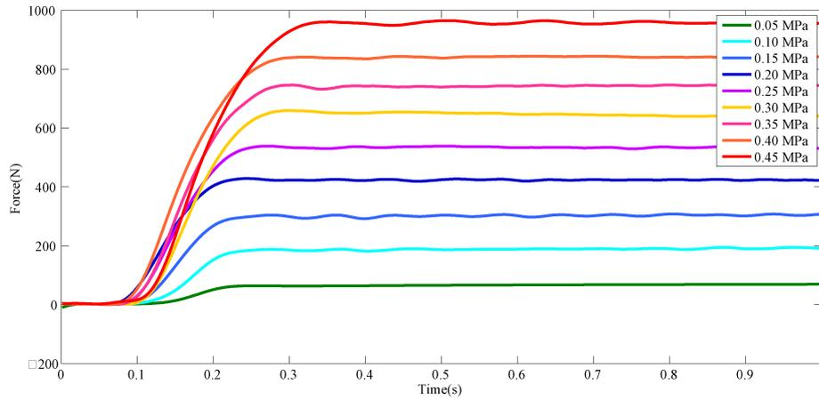
Figure 2.5: Dynamic Characterization of Pneumatic Muscle Actuator: scale at the range of one second.
