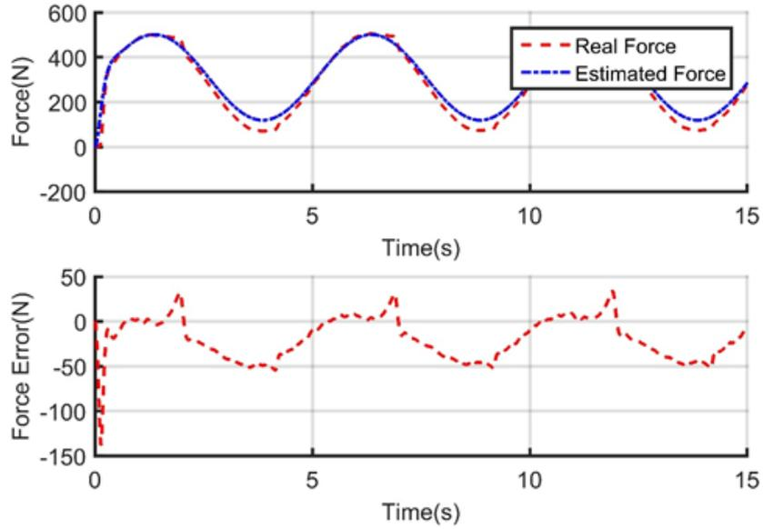
Figure 4.3: Comparison between the estimated force from model and the measurement force from muscle at frequency 0.2 Hz.
