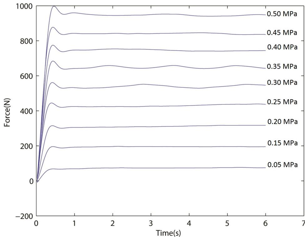
Figure 2.4: Dynamic Characterization of Pneumatic Muscle Actuator.
