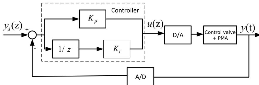
Figure 4.9: Block diagram of the PID controller.
