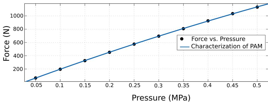
Figure 2.3: Pneumatic muscle characterization: The Force-Pressure relationship.
