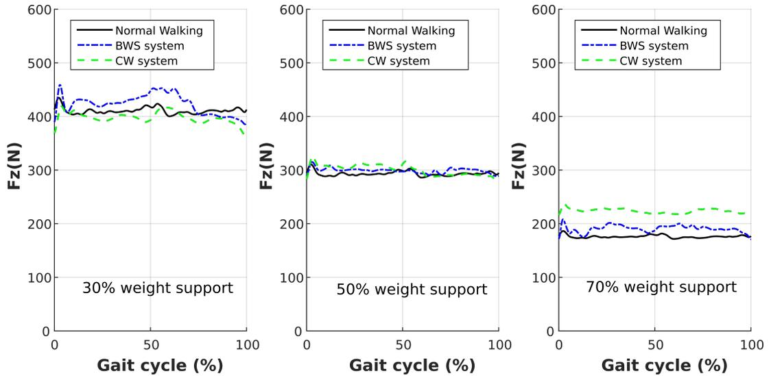
Figure 5.8: Reaction Force When applying Weight systems. Backline Reaction Force at 0% is scaled for comparison, Blue Reaction force using the Active system, Green Reaction force using Counter Weight system. From the left to the right, the weight support level is 30%, 50%, and 70%, respectively.
