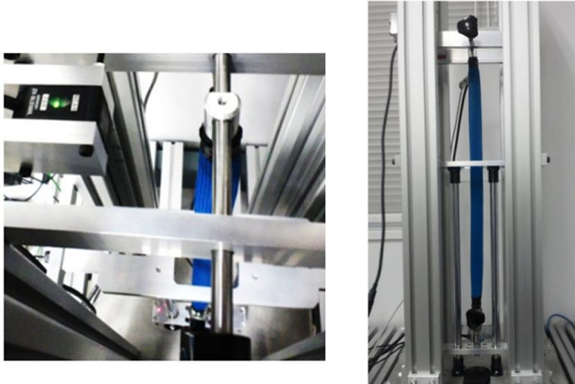
Figure 2.2: The Testbed used for conducted experiments to investigate the characteristic of the pneumatic muscle actuator.
