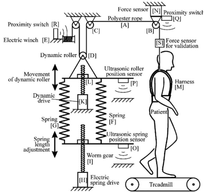
Figure 1.3: The novel mechatronic BWS system using the complicated rope-pulley-spring system [24].
