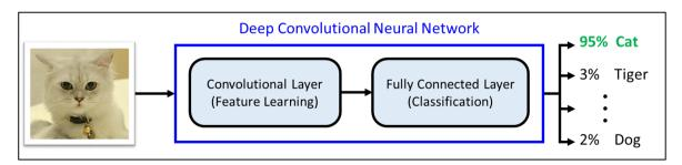
Figure 7.1 Deep Convolutional Neural Network Architecture
