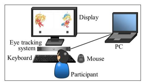
Figure 3.4 Experimental setup where participant looks at illustrations on PC monitor while eye tracking system records his eye movements
