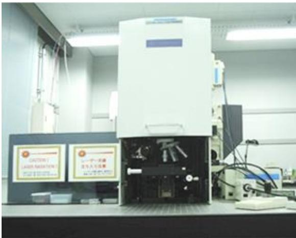
*Figure 3.5 Micro Raman Spectrometer*
