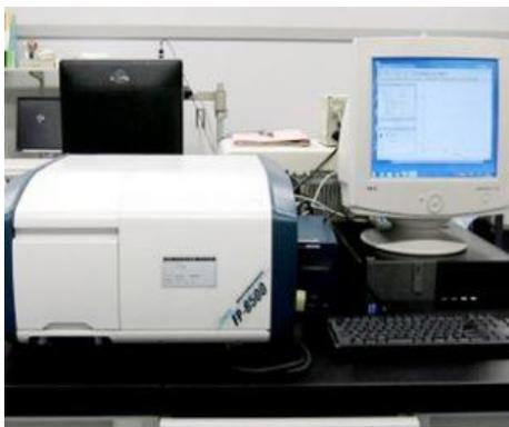
*Figure 3.6 Fluorescence Spectrometer*
