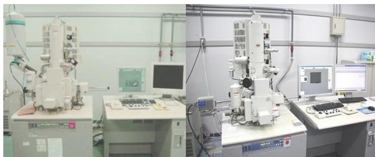
*Figure 3.7 FESEM EDX S-4800 EDX, (HORIBA) and Hitachi FE-SEM SU8000, EDX (Bruker)*
