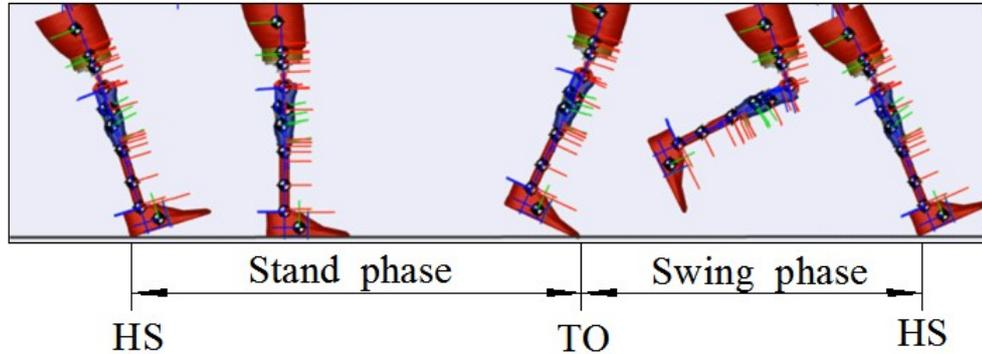
Figure 4.16: Gait cycle in simulation .
