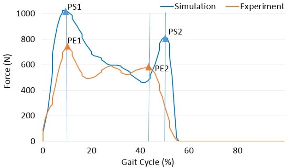
Figure 5.4: Vertical ground reaction force by simulation and measurement.
