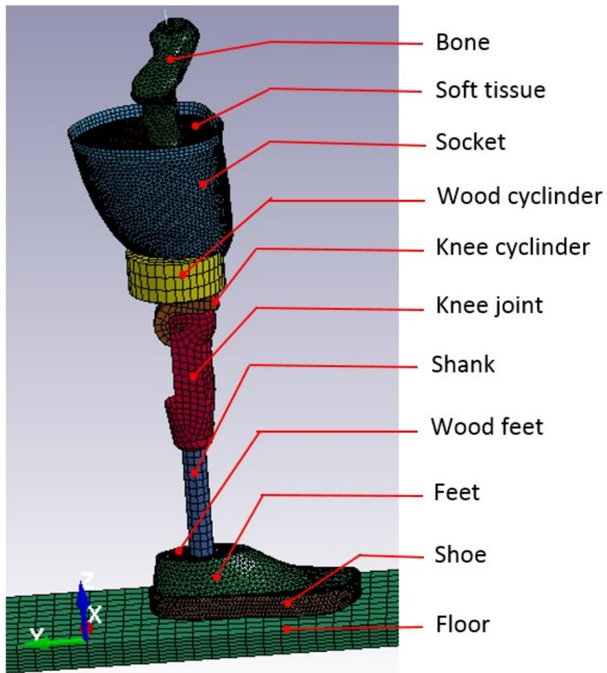
Figure 5.3: Finite element model of the residual limb with a transfemoral prosthesis.
