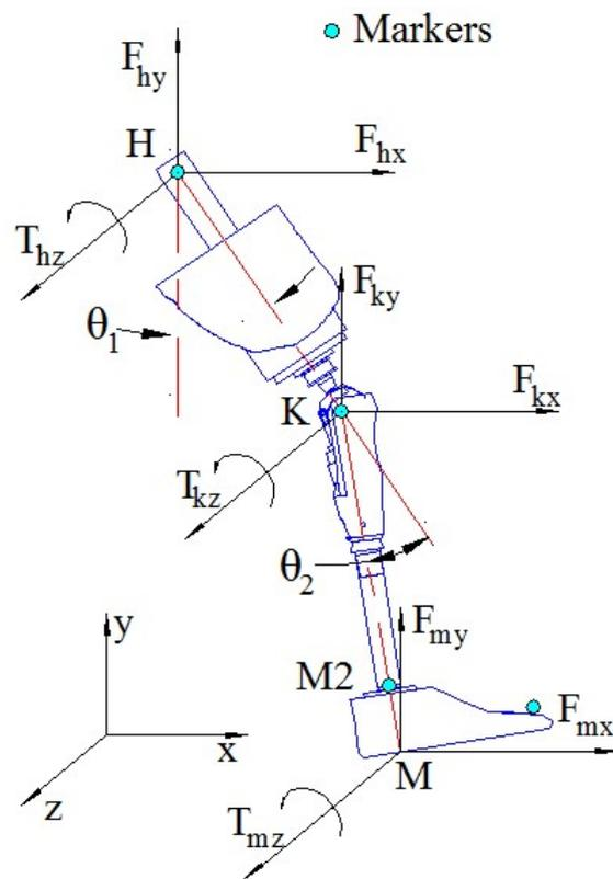
Figure 4.6: Position of markers and angles on lower limb.
