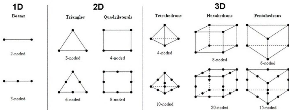
Figure 2.2: Different 1D, 2D and 3D basic elements
