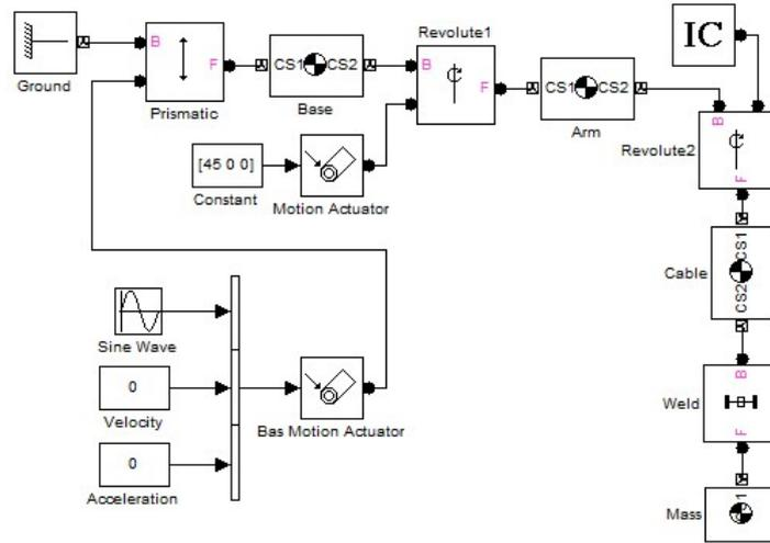
Figure 2.7: Example of Simmechanics Block Diagram (Matworks Inc).
