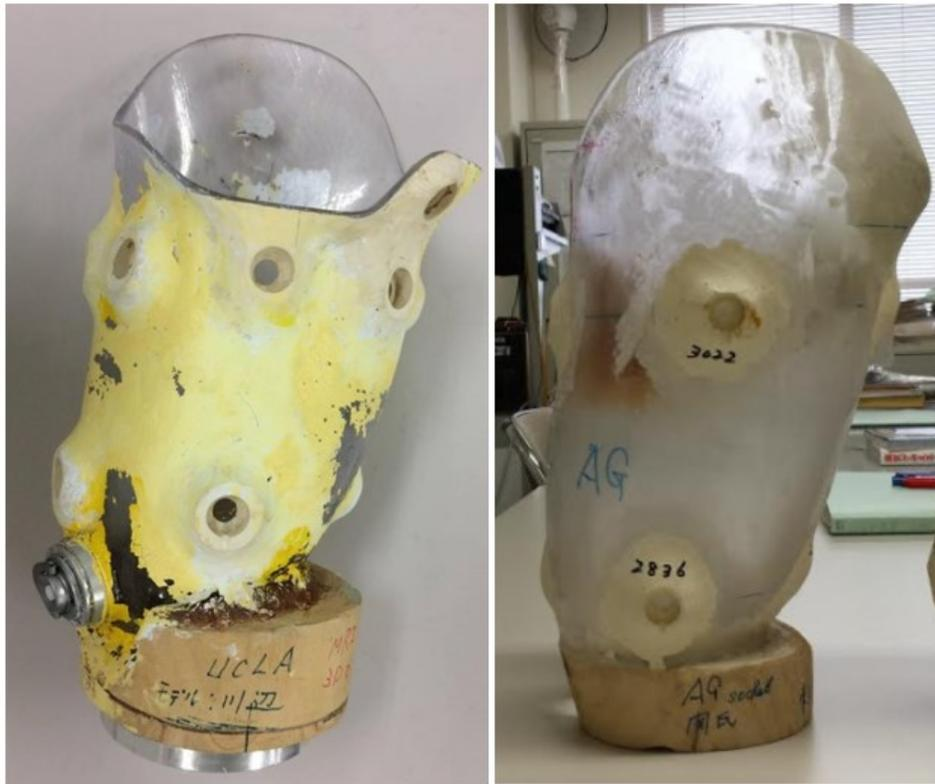
Figure 1.4: The UCLA socket type and MCCT socket type. Made by prof. Agarie laboratory.
