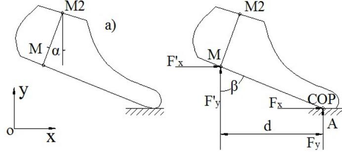
Figure 4.10: Schema for calculating position and load at M point.
