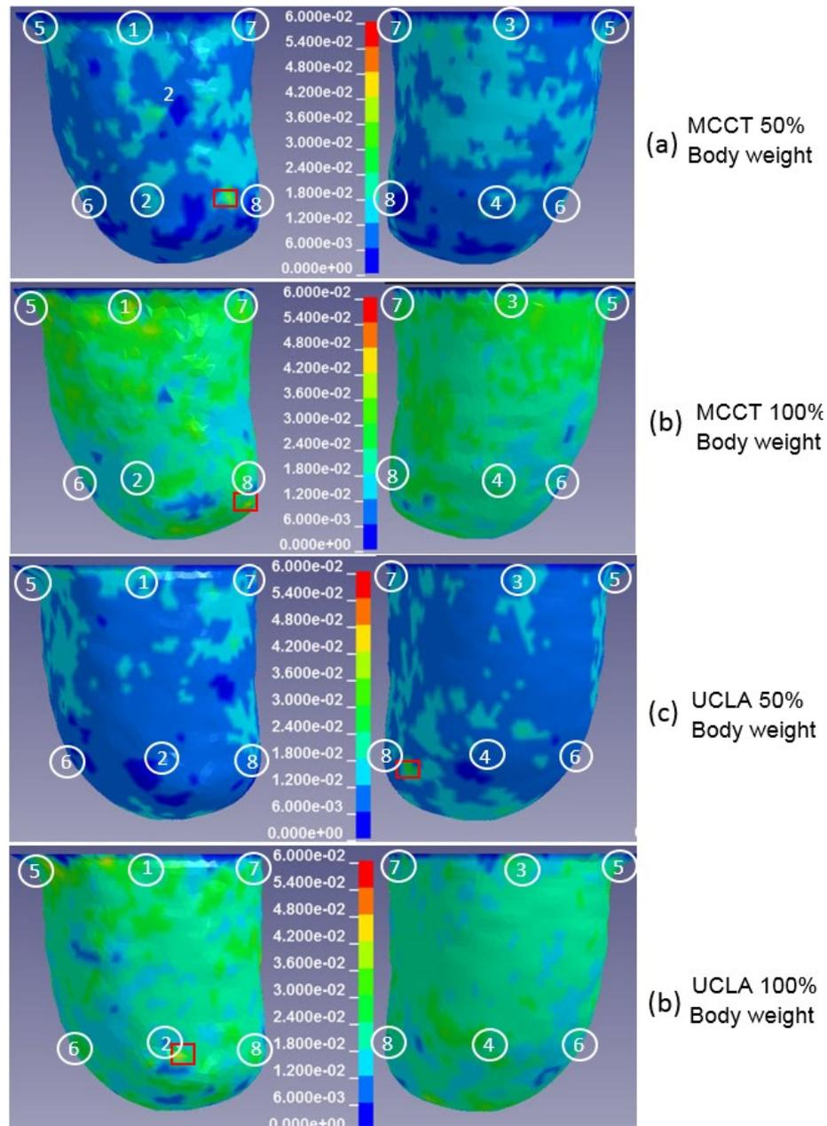
Figure 3.11: Distribution of interface pressure (Unit: MPa). Anterior (left side) and posterior (right side) view. Red rectangles show positions where the maximum pressure is observed on residual limb. White circles 1, 2, 3, 4, 5, 6, 7, and 8 show the position of sensors at AP, AD, PP, PD, MP, MD, LP, and LD, respectively.
