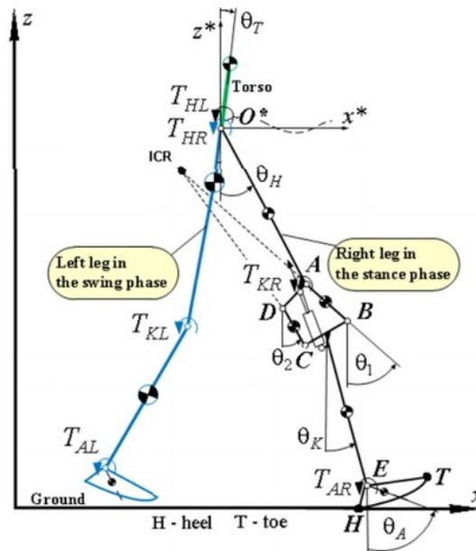
Figure 2.9: Kinematic scheme of human walking with prosthesis with the polycentric artificial knee joint mechanism [72].
