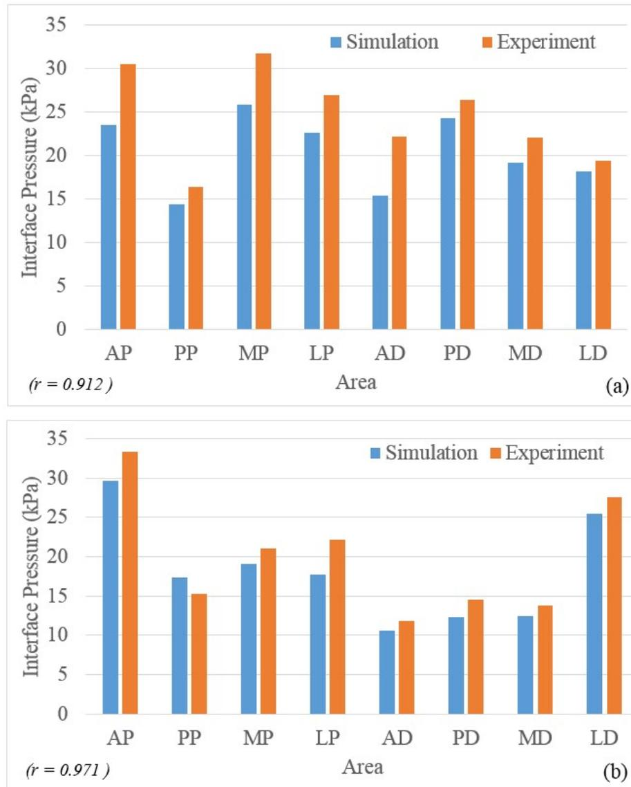
Figure 3.9: The value of pressure at sensors location in the experiment and simulation in case of MCCT (a) and UCLA (b) socket with 50 percent body weight.
