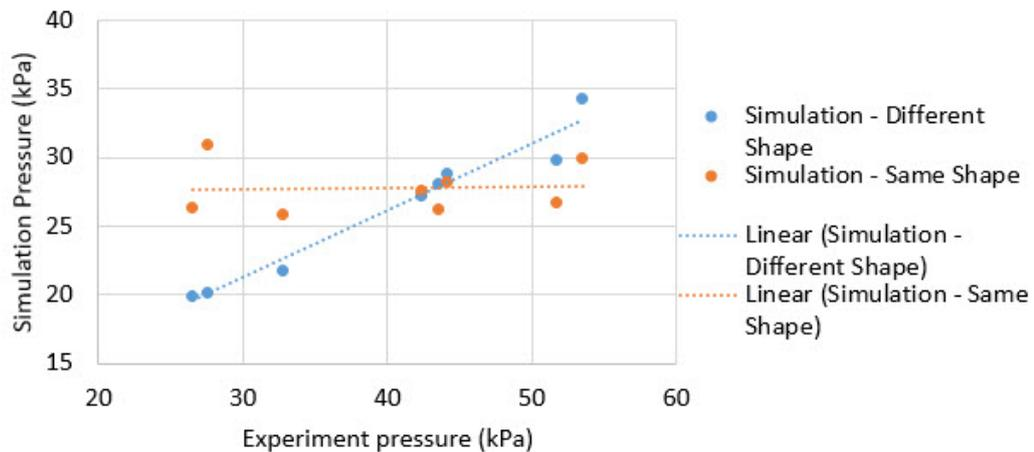
Figure 3.8: The scatter diagram shows the relation between experimental results and two cases of simulation results.
