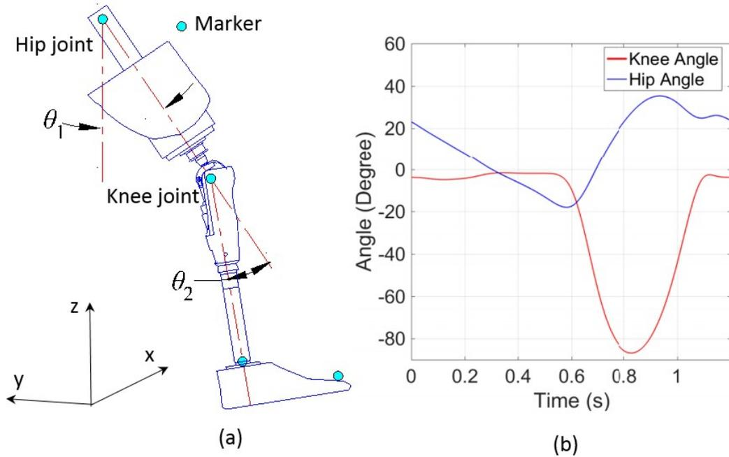
Figure 5.2: (a) Diagram of the rotation of the hip and knee joints and (b) rotational angles of the hip and knee joints.
