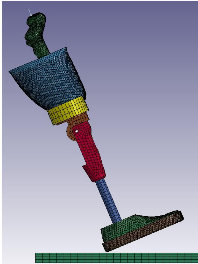
Figure 4.21: The finite model of the prosthesis.
