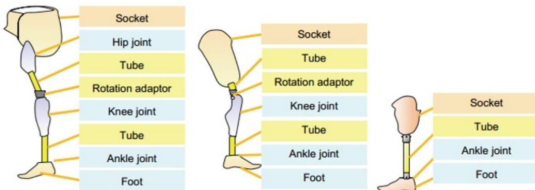
Figure 1.2: Main components of the lower limb prosthesis (NRCD Japan). Hip prosthesis (left); Transfemoral prosthesis (middle) and Transtibial prosthesis (right)
