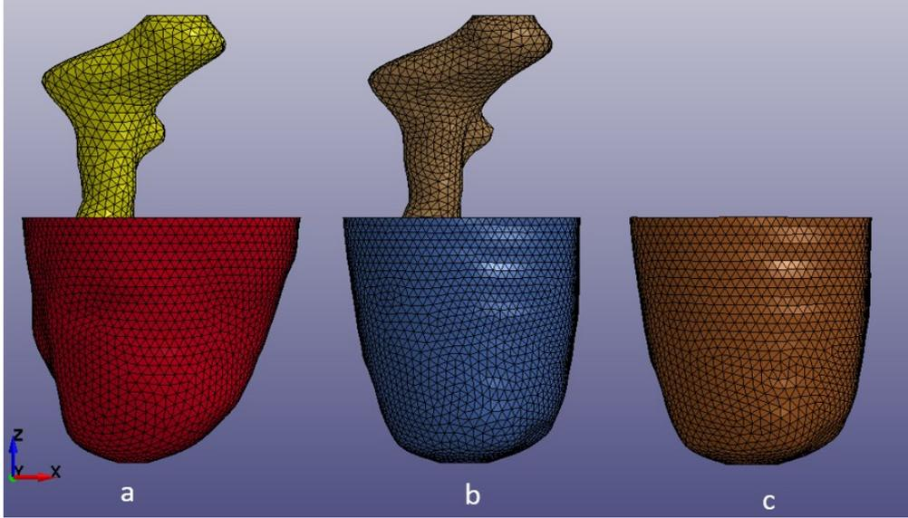
Figure 3.4: The FE model of residual limb in case of different shape with MCCT socket (a); same shape with MCCT socket (b) and the socket (c).
