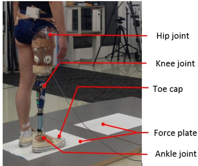
Figure 5.1: Marker positions on the subject and force plates during the experiment.
