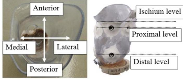
Figure 3.6: The position of eight sensors on socket
