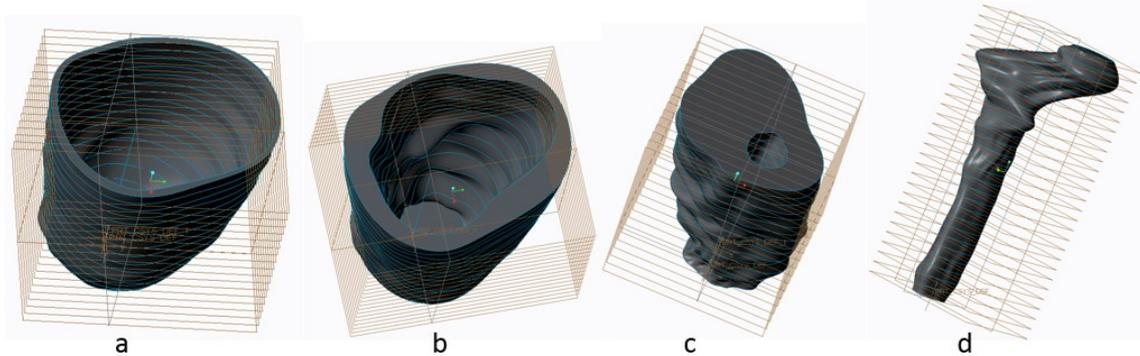
Figure 3.3: 3D model of parts of residual limb. (a. Skin; b. Fat; c. Muscle; d. Bone).
