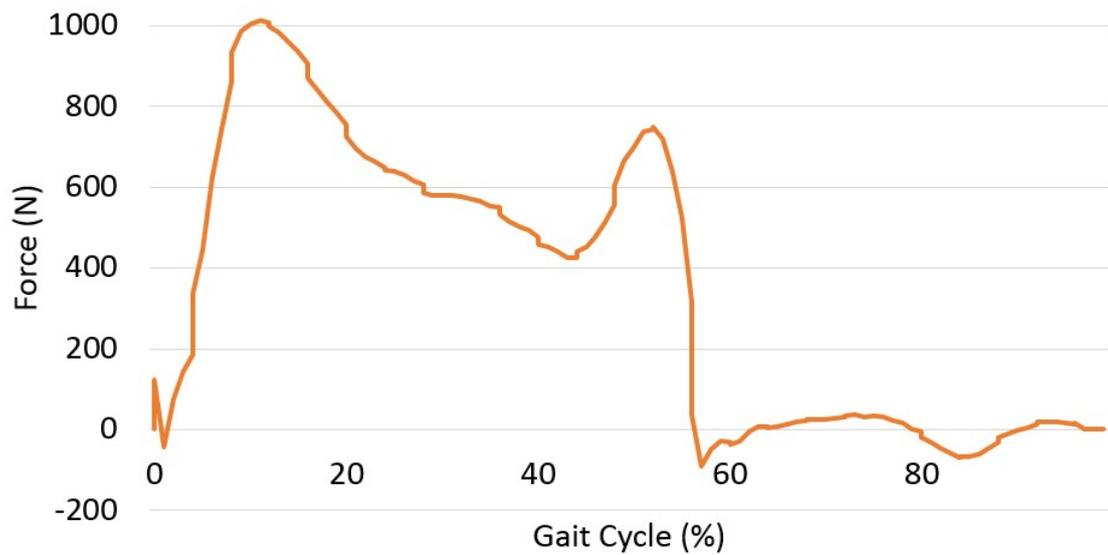
Figure 5.5: Vertical reaction forces at the knee joint.
