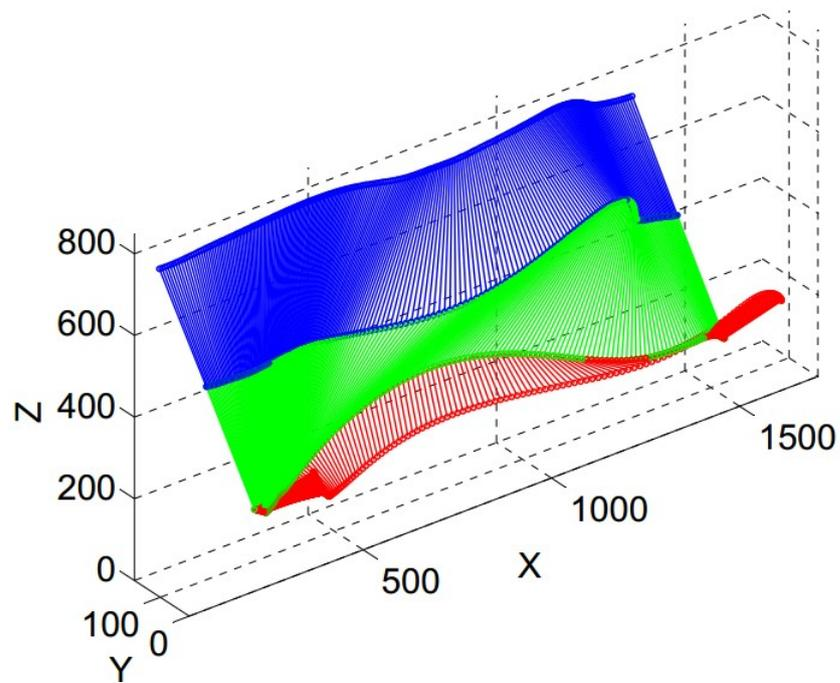
Figure 4.5: Schema movement of lower limb with prosthesis (mm).
