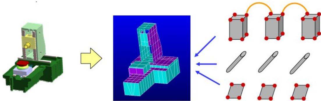
Figure 2.1: Divide the domain into a number of small, simple elements (MIT web)
