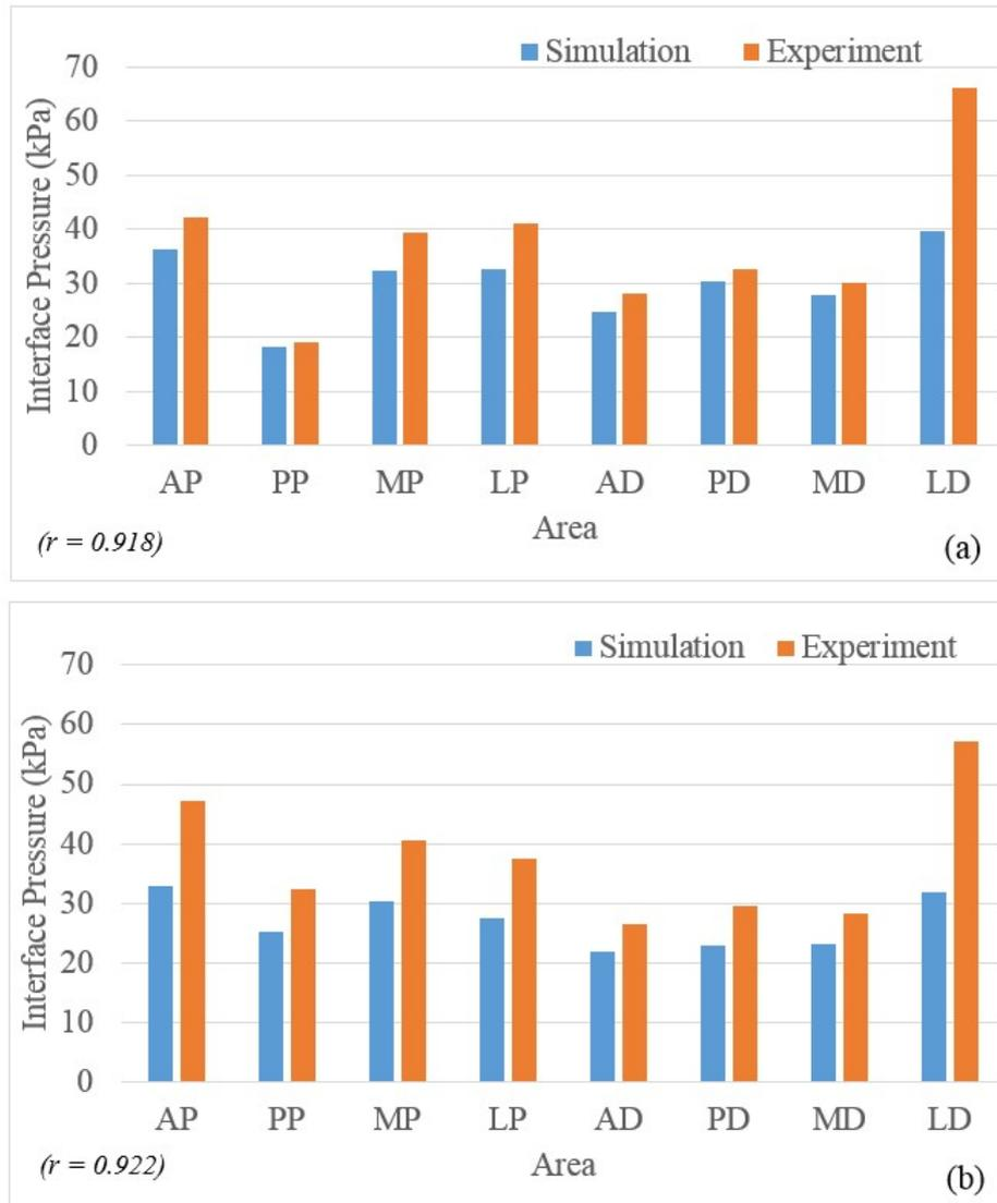
Figure 3.10: The value of pressure at sensors location in the experiment and simulation in case of MCCT (a) and UCLA (b) socket with 50 percent body weight.
