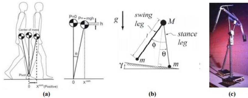
Figure 2.8: Simple models of human gait. (a) Inverted pendulum model [50]. (b) 2D passive walking [43]. (c) Cornell 3D passive biped with arms [33].
