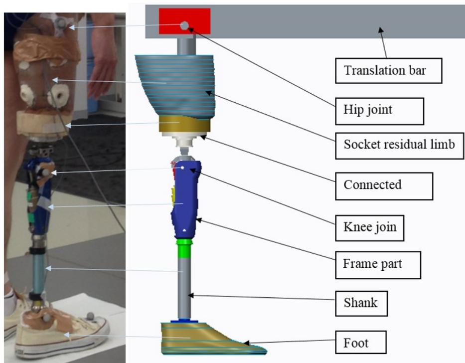
Figure 4.9: The actual and 3D model of lower limb with prosthesis.
