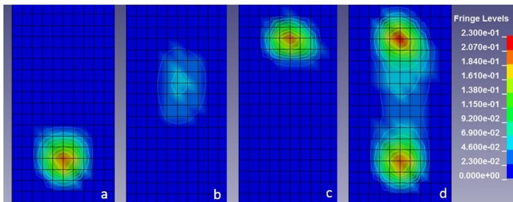
Figure 5.6: Distribution of the interface pressure between the shoe sole and floor at the (a and c) first and second vGRF peaks, (b) midstance, and (d) at the sum of all the states in the stance phase.
