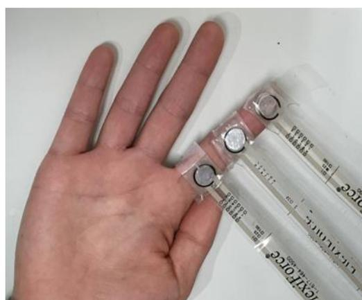
**Figure 14 Placement of force sensor to right hand of index finger**
