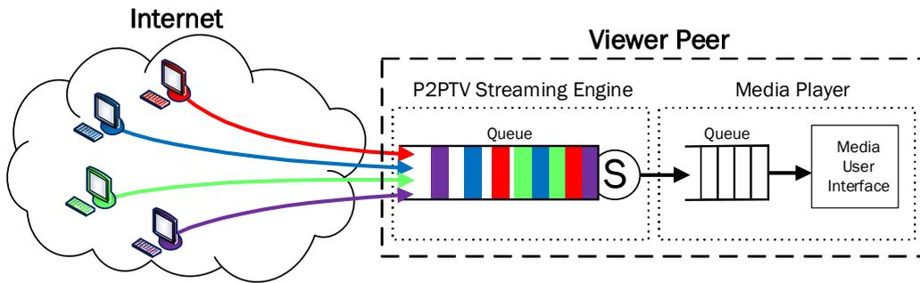
FIGURE 2.5: Streaming process of user device installed P2PTV application.
