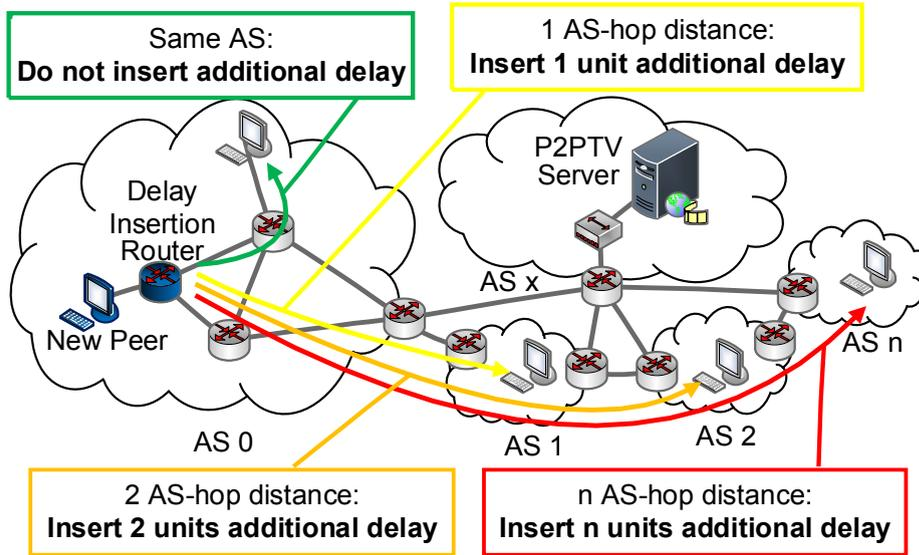
FIGURE 3.1: Conceptual illustration of delay insertion related to AS hop distance.
