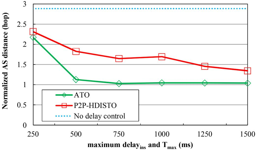
FIGURE 4.7: Normalized AS hop distance versus amount of delay insertion in SopCast application.
