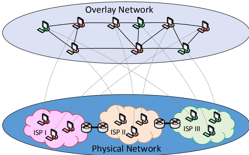
FIGURE 2.6: Connection of peer on overlay network without physical network consideration.
