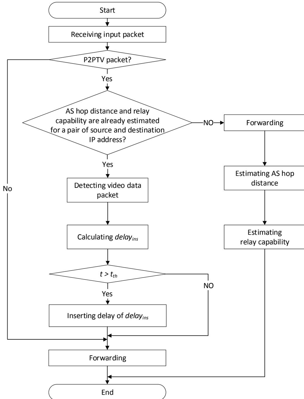
FIGURE 5.5: Flow chart of delay insertion into P2PTV packet by the proposed LoRCAD scheme.
