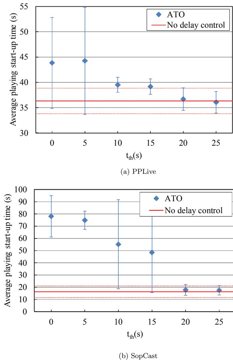
FIGURE 4.2: Effect of varying starting time for delay insertion ( $t_{th}$ ) on the playing start-up time in P2PTV applications.
