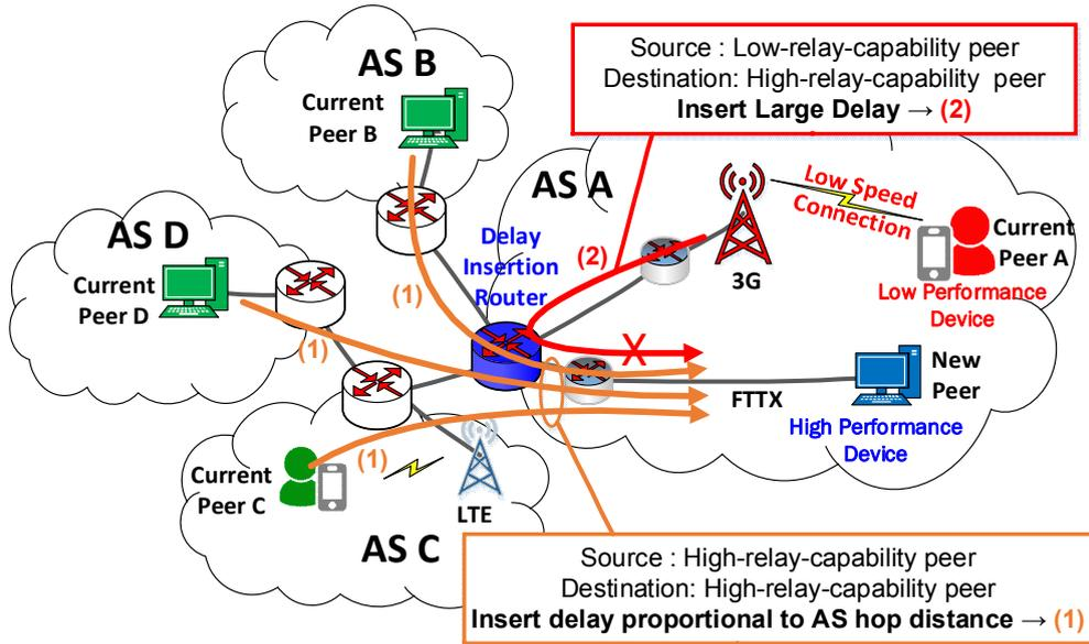
FIGURE 5.2: Operation of the delay insertion router when detecting the high-relay-capability peer.
