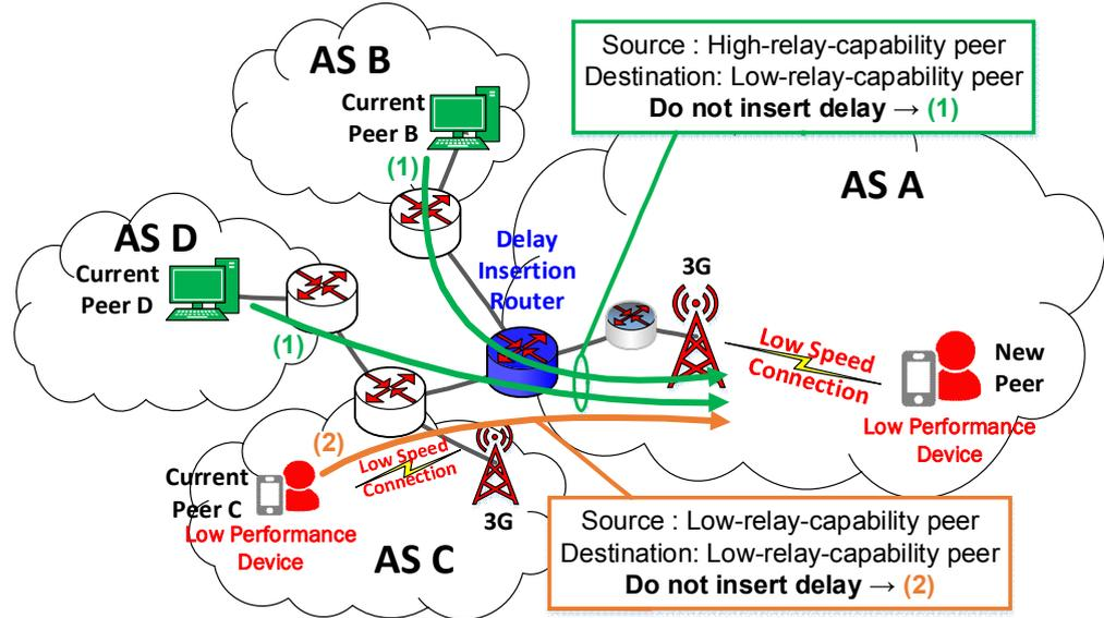
FIGURE 5.3: Operation of the delay insertion router when detecting the low-relay-capability peer.
