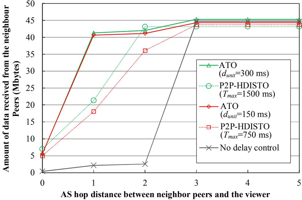
FIGURE 4.6: Cumulative amount of data received for SopCast application.
