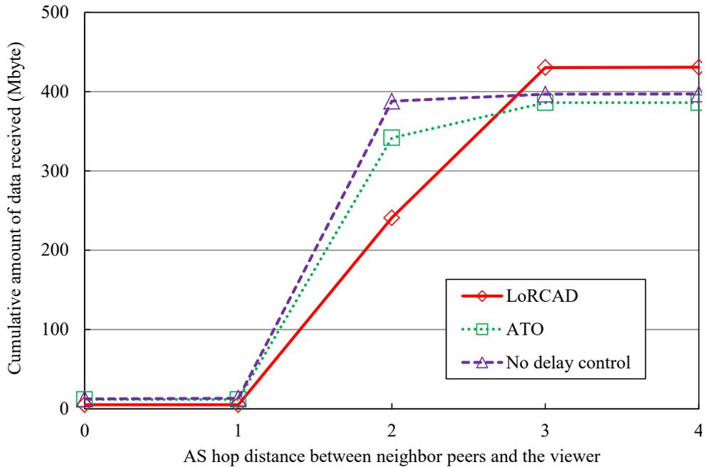
FIGURE 6.12: Cumulative amount of data received by the low-relay-capability peer in PPLive application.
