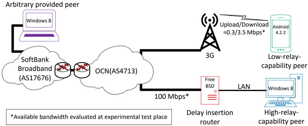
FIGURE 6.1: Experimental setup for LoRCAD scheme evaluation.
