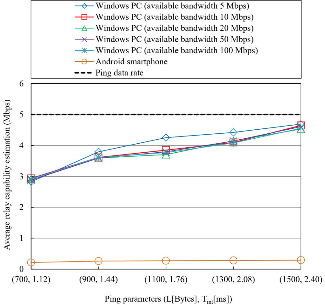
FIGURE 6.2: Estimated relay capability when using ping datarate 5 Mbps.
