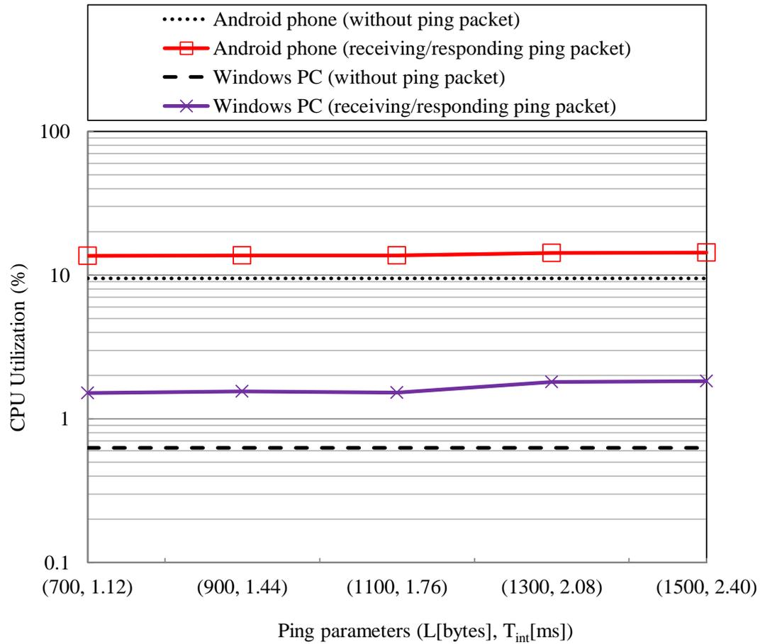
FIGURE 6.3: Effect of ping parameters on CPU utilization.
