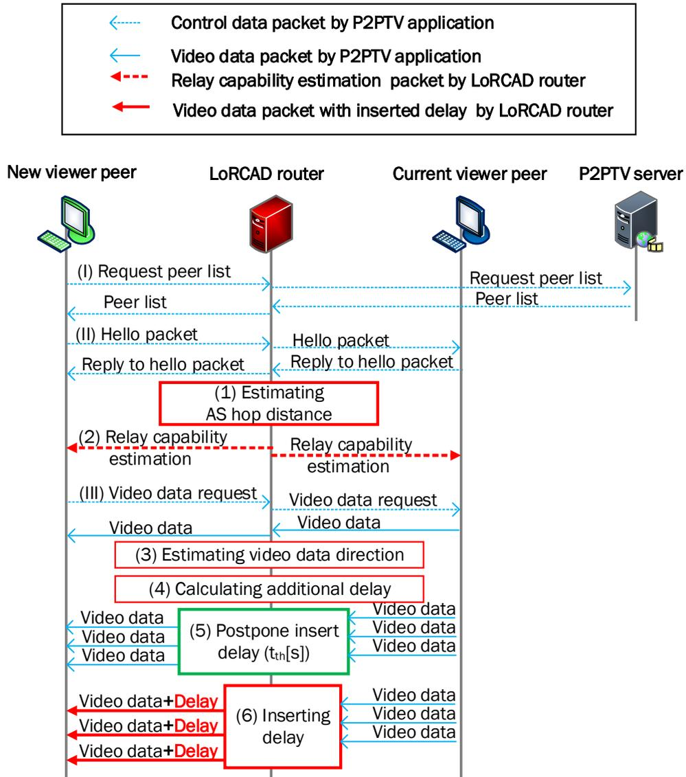
FIGURE 5.4: Time sequence of the LoRCAD Scheme when deployed to P2P application.
