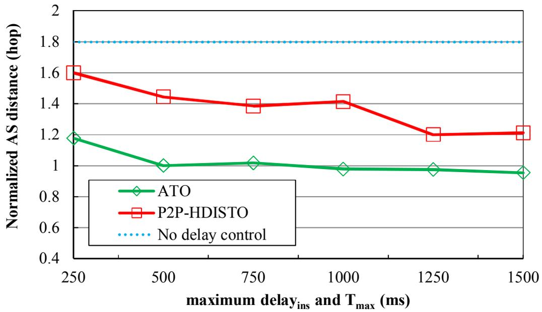
FIGURE 4.4: Normalized AS hop distance versus amount of delay insertion in PPLive application.
