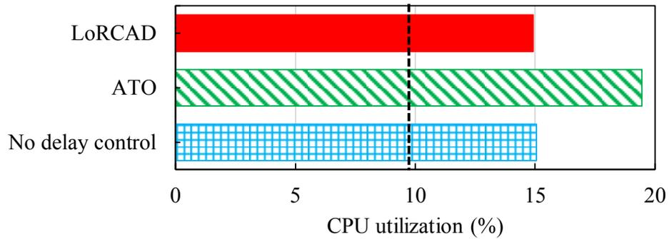
FIGURE 6.5: CPU utilization at the local low-relay-capability upstream peer while deployed traffic localization schemes.
