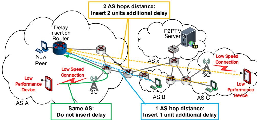
FIGURE 5.1: Limitation of ATO scheme which insert delay proportional to AS hop distance without relay capability consideration.
