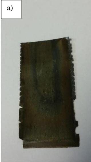
Figure 4. 7: 100Ni:50Ti:100Ni before annealing.
