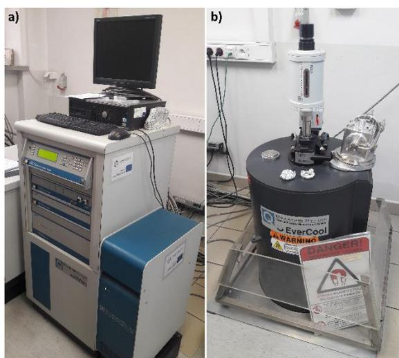
Figure 2. 9: Images of Physical Properties Measurement System with 9 T superconducting magnet: a) PC with PPMS electronics cabinet and b) Dewar/probe (with mounted VSM module, Quantum Design).
