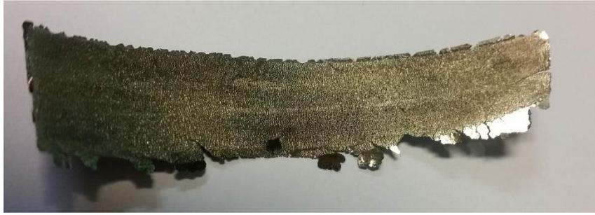
Figure 4. 9: The image of foils after secondary cold rolling of cold rolled heated foils.
