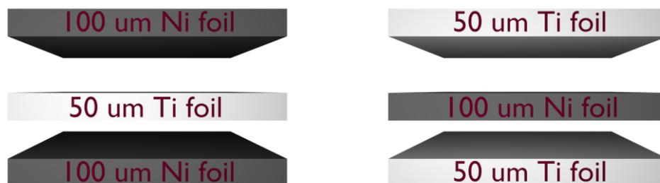
Figure 4. 1: Illustrative representation of the cold rolled diffusion couples: a) 50  $\mu\text{m}$  titanium foil between two 100  $\mu\text{m}$  nickel foils and b) 100  $\mu\text{m}$  nickel foil between two 50  $\mu\text{m}$  titanium foils.
