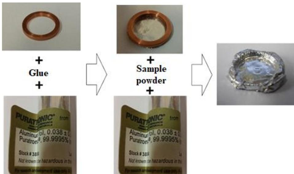
Figure 2. 7: Mössbauer Spectroscopy sample preparation process.
