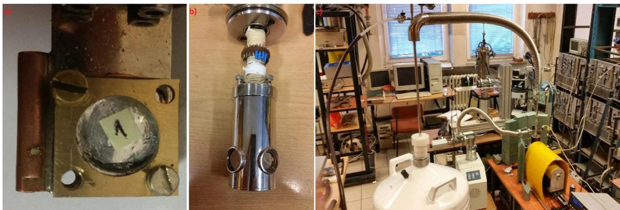
Figure 2. 8: a) Sample inside holder, b) gas flow cryostat and c) Mössbauer Spectroscopy measurement setup.
