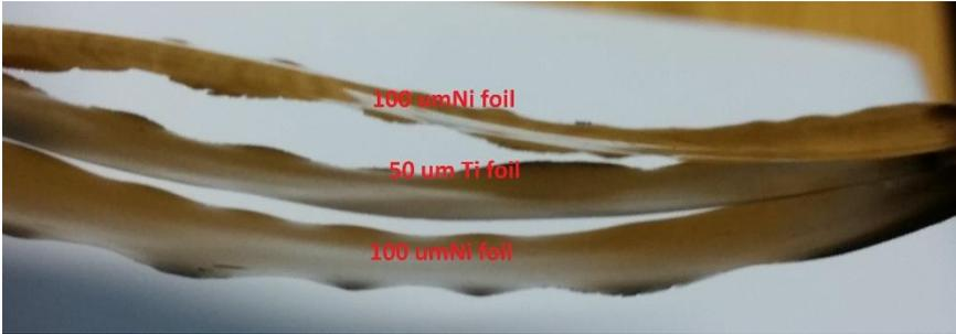
Figure 4. 8: The image of foils cold rolled without prior heating treatment.
