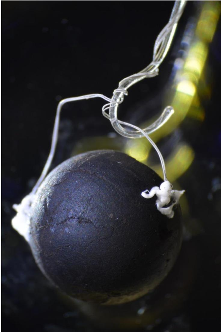
**Figure 4.3** Sample of 10 mm ready for the test (white adhesive agent visible on sides).
